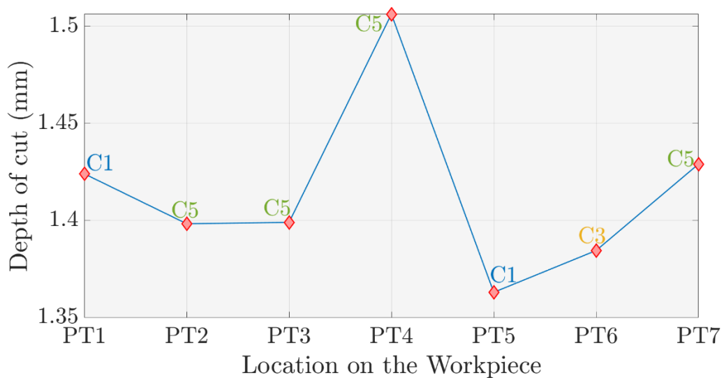
Figure 4-9: Configuration identification based on maximum stability along the tool path at 16100 rpm
