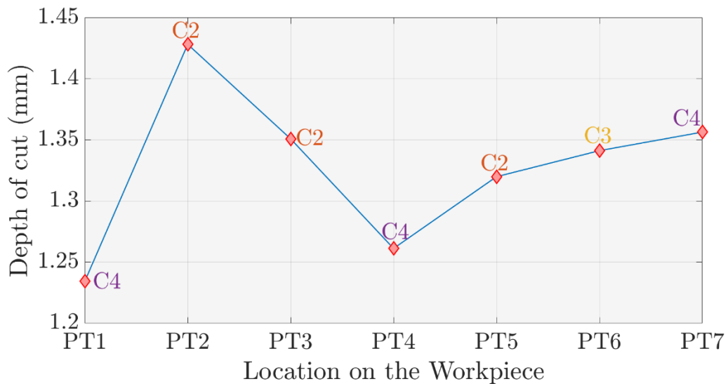
Figure 4-13: Representative plot on maximum stability along the tool path regarding constant spindle speed at 15920 rpm & limited configuration variation between C2—C4 in X direction
