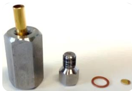
Figure 2-3 Stainless steel reactor (autoclave) and its components, used in the synthesis process.
