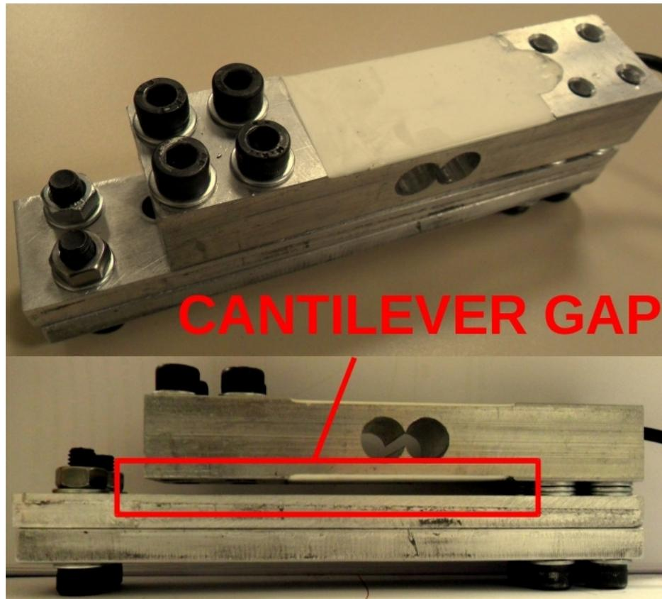
Figure 3.10: Manufactured cantilever for compression force calibration.
