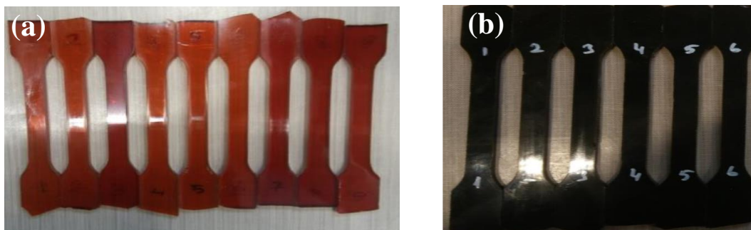
Figure 4.2 The prepared (a) reference and (b) TEGO reinforced tensile test specimens.
