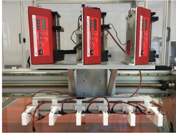
Figure 3.3 Completed assembly of the pump stand.
