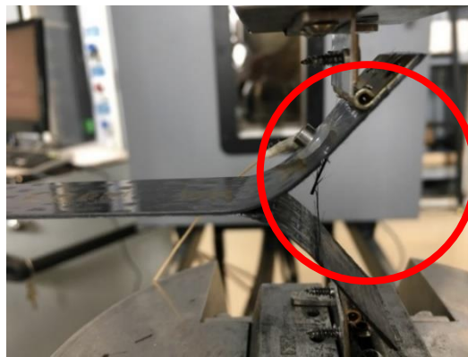
Figure 2.15 Fiber bridging during mode I fracture toughness test.
