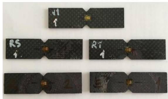
Figure 4.21 Damaged test specimens after completing the shear tests.
