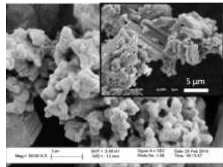
d) SEM micrograph Nb 2 O 5 powder (orthorhombic+ monoclinic)
