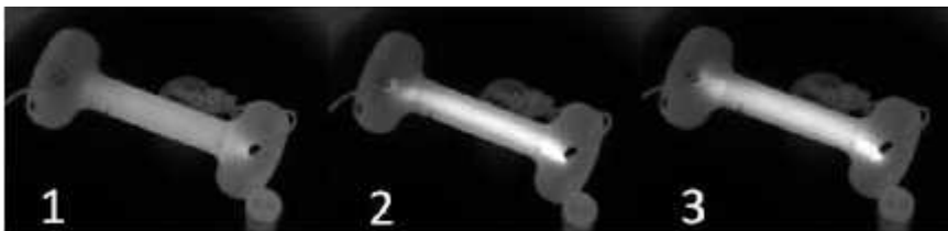
Fig. 4.2. Images of the sample before the flash, initiation of flash and during flash sintering.
