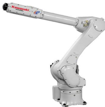
FIGURE 3.2: Six axis articulated robot [96]
