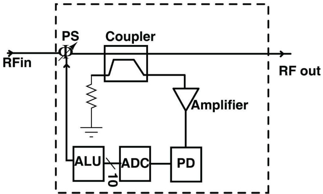
Fig. 47: Block diagram of the second prototype consisting of completely integrated RF and baseband building blocks.
