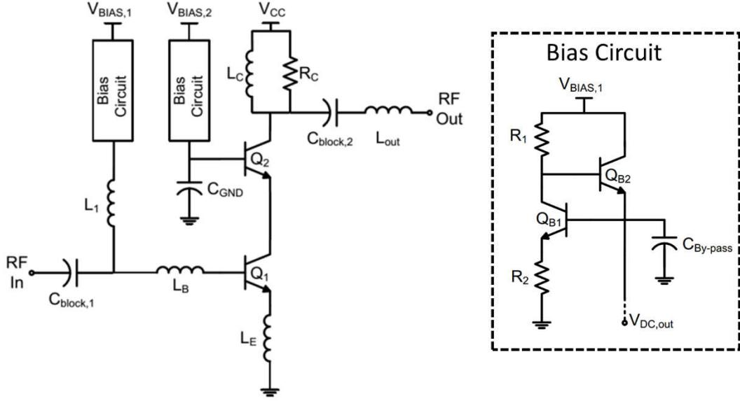
Fig. 29: Schematic of amplifier circuit.
