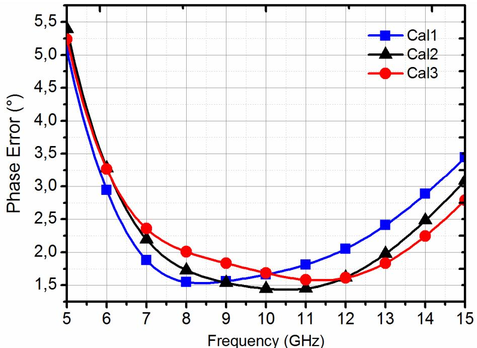
Fig. 42: Simulation results for the comparison of rms phase error of three calibrations. In Cal1, Cal2 and Cal3 calibration signals are sent at 9, 10 and 11 GHz, respectively.
