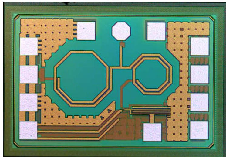
Fig. 24: Die photo of the power detector. Total chip area is 0.42 mm<sup>2</sup>, including the pads.
