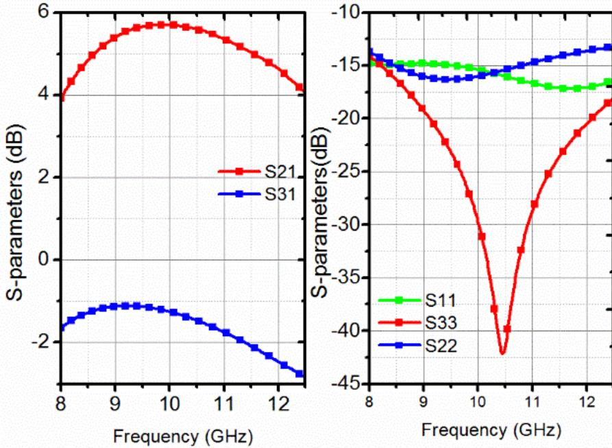
Fig. 39: S-parameter simulation results of the RF circuits before PD, S<sub>21</sub> is the gain at calibration path, S<sub>31</sub> is the insertion loss at signal path, S<sub>11</sub> is the input RL, S<sub>22</sub> is the output RL at calibration path, S<sub>33</sub> is the output return loss at signal path.
