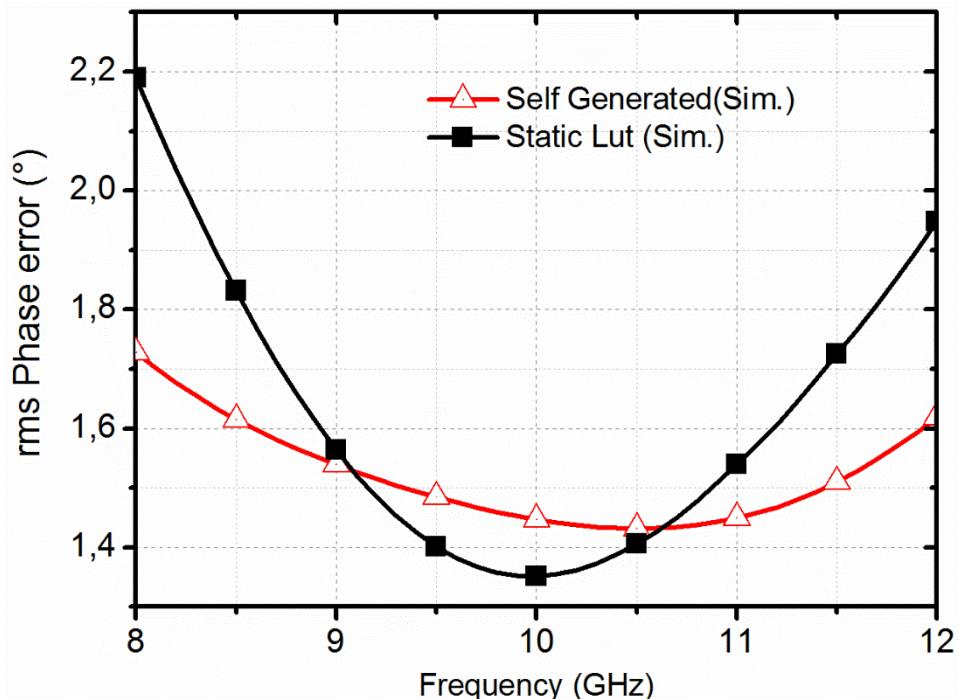
Fig. 43: Effect of the calibration on rms Phase error in process corners – Best Case.
