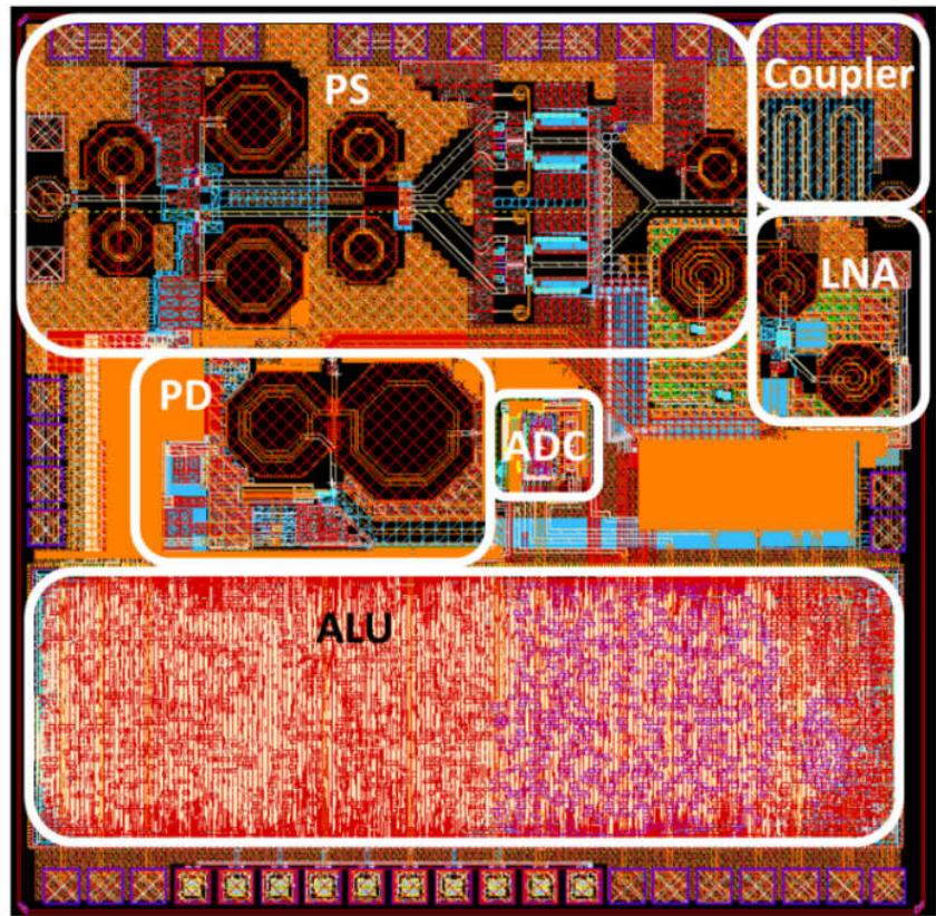
Fig. 48: Layout of the final circuit.
