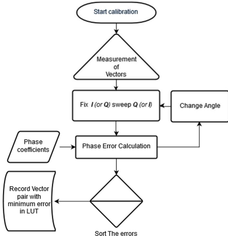
Fig. 36: Flowchart of the proposed digital processing unit.
