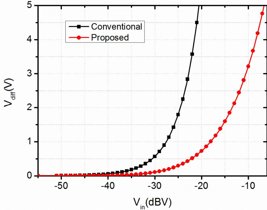
Fig. 23: Theoretical comparison of conventional PD and proposed PD.
