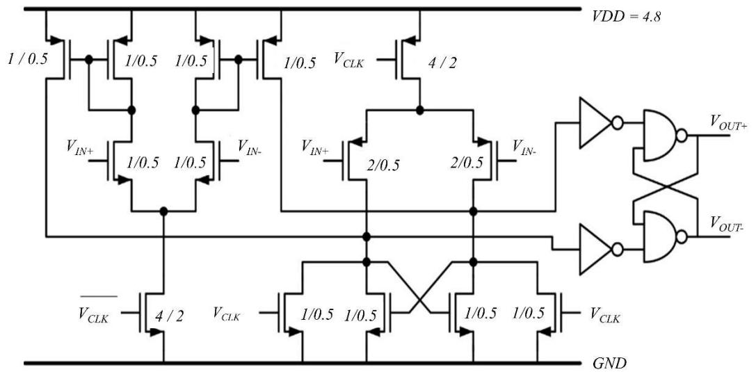
Fig. 33: Comparator circuit with optimized transistor geometries.
