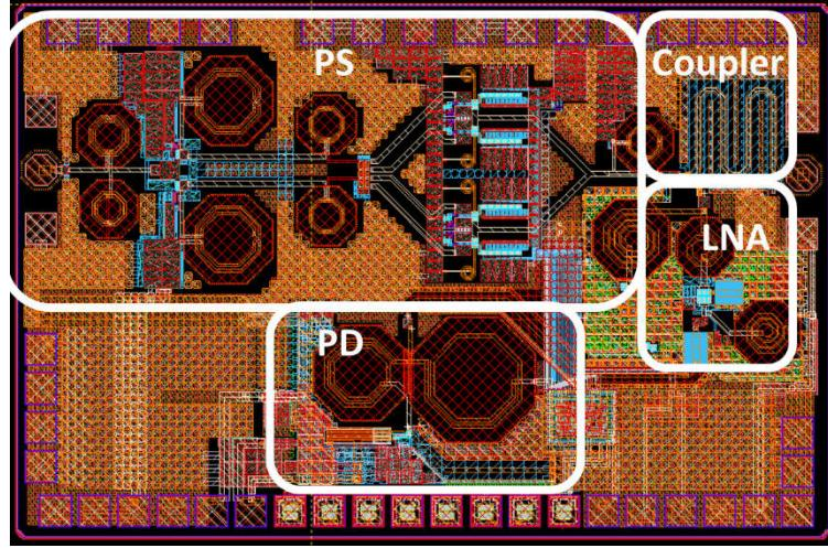
Fig. 38: Layout of the first prototype
