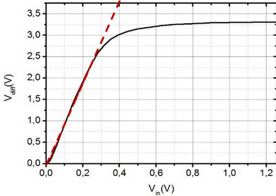
Fig. 25: Output DC voltage vs input signal amplitude. Dashed line shows the linear region.
