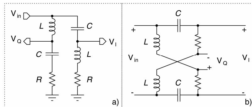
Fig. 10: L-C resonance-based quadrature all pass filters (LCQAF), a)Single ended, b) differential.
