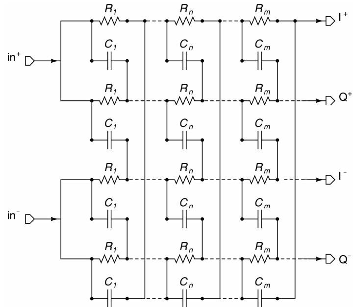
Fig. 9: Polyphase filter as a quadrature generator.
