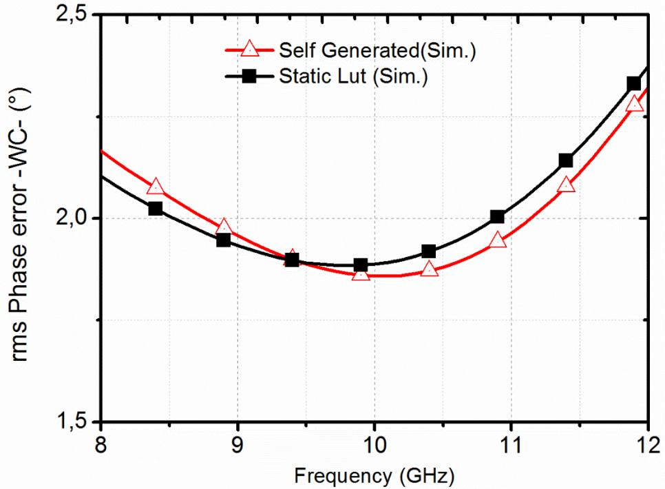
Fig. 44: Effect of the calibration on rms Phase error in process corners – Worst Case.
