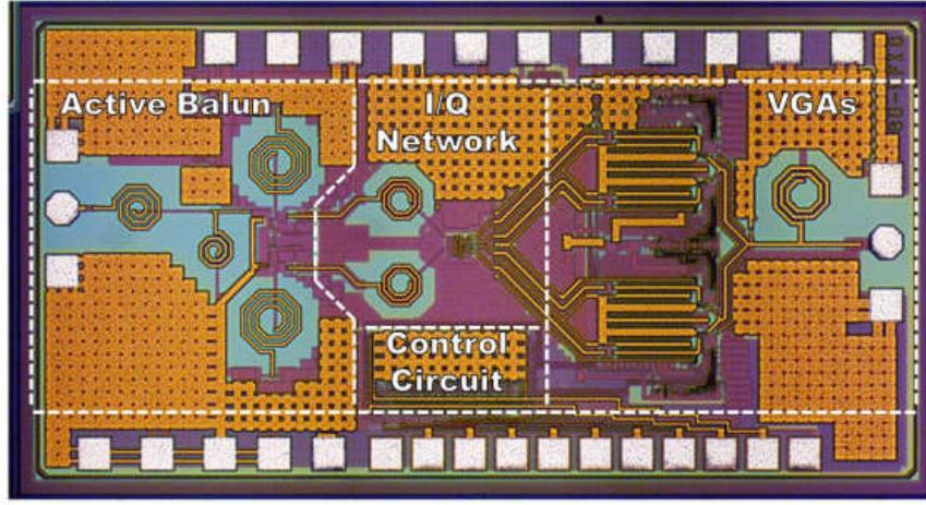
Fig. 19: Die photo of previously fabricated vector sum based phase shifter with static LUT.
