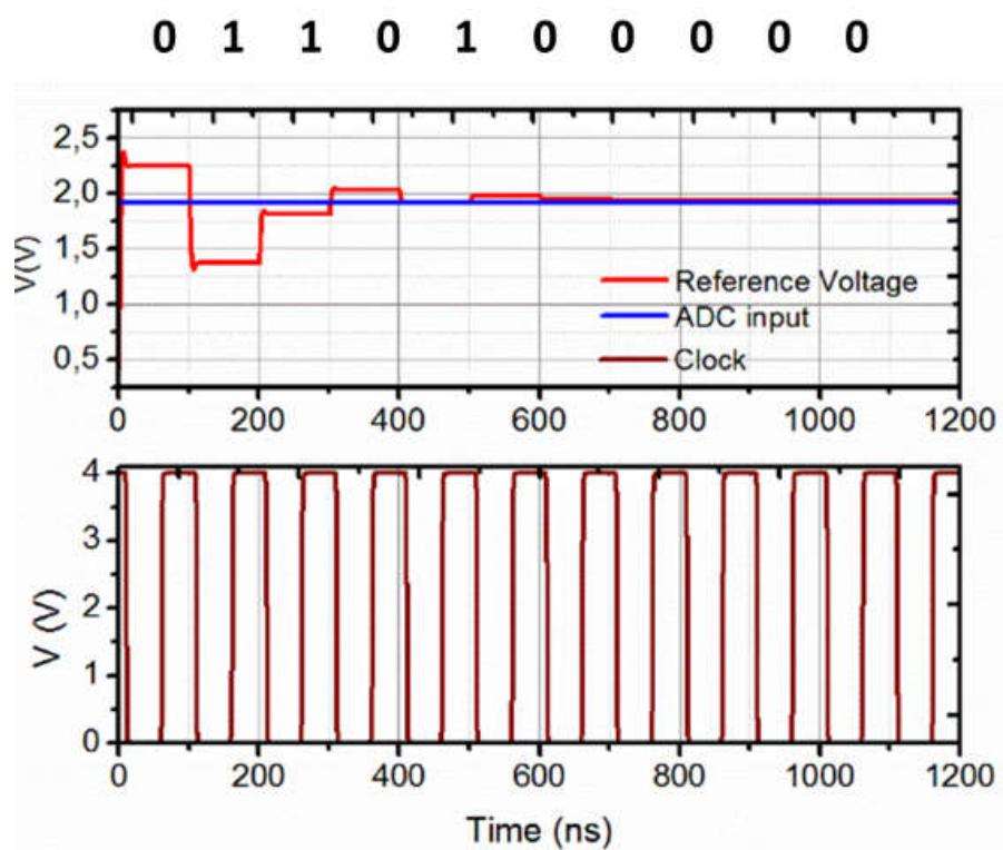
Fig. 34: Post layout transient Simulation Results of ADC.
