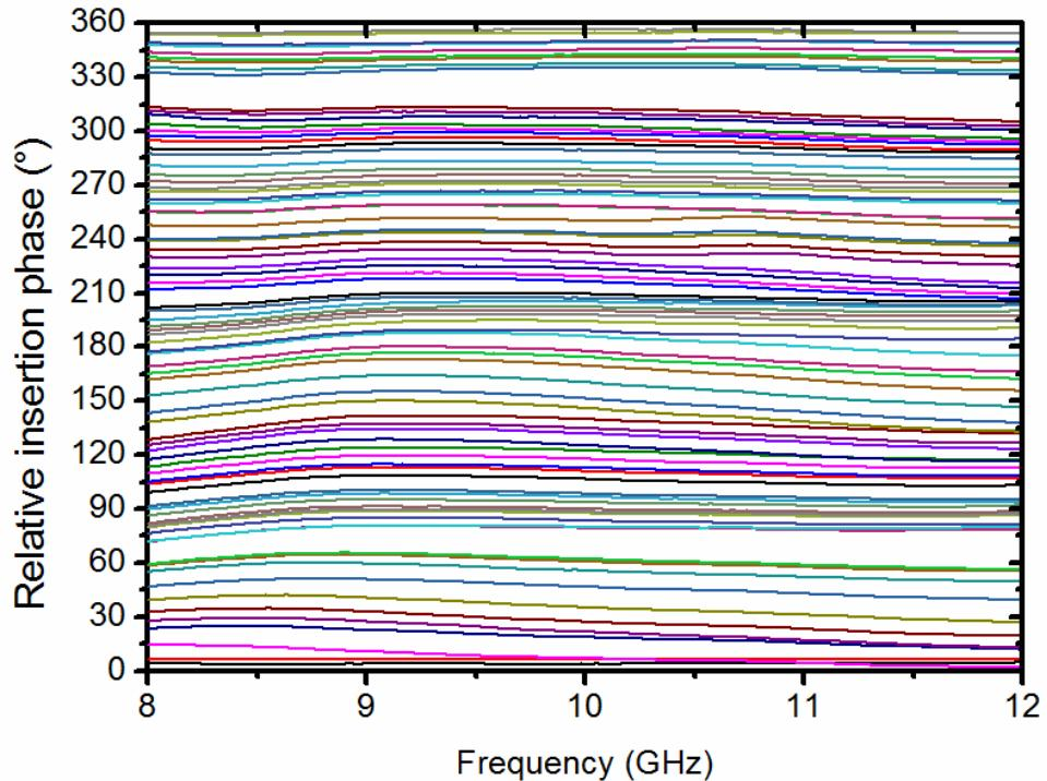
Fig. 54: Measured relative insertion phase response of PS with *Static LUT* which is based on post layout simulation results.
