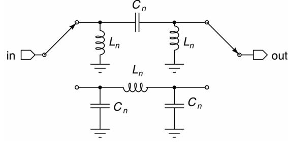
Fig. 4: High-pass/Low-pass phase shifter.
