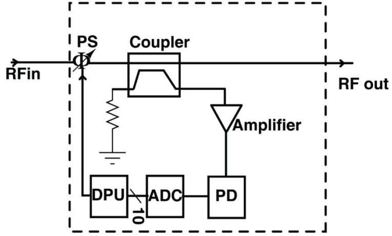
Fig. 13: Block diagram of the proposed self-calibration circuit.
