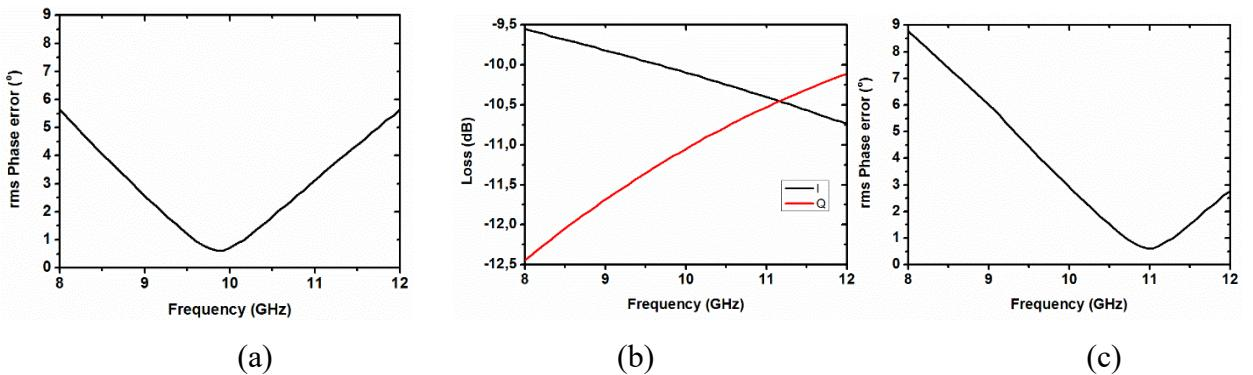
Fig. 8: a) rms phase error with using an RC-CR network at [56] b) simulation result for S21 variation after 1 dB gain improvement at I path, c) rms phase error after this improvement.
