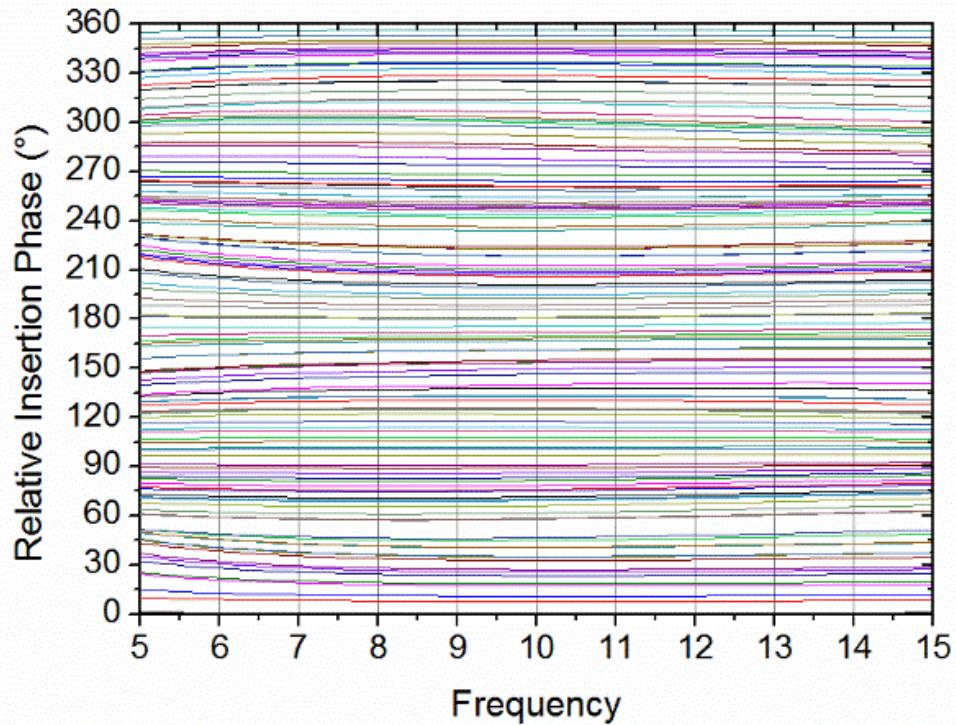
Fig. 40: Relative insertion phase response of phase shifter after calibration.
