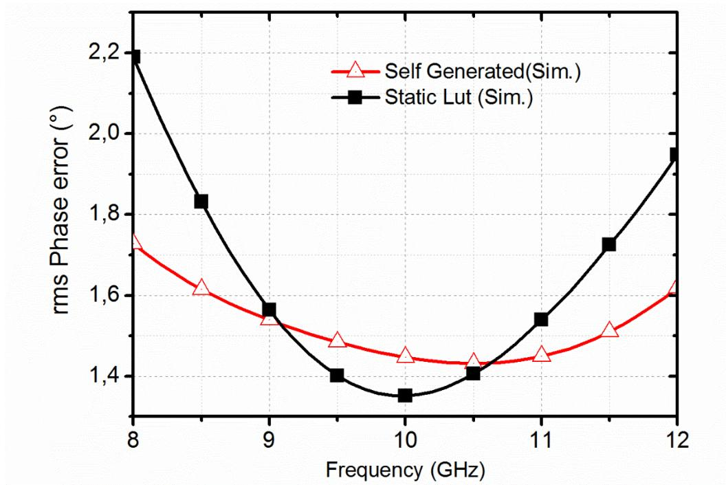
Fig. 41: rms Phase error of phase shifter with and without calibration for typical conditions.
