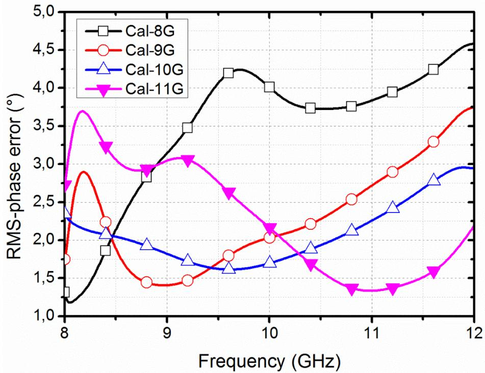
Fig. 60: Measurement results for the comparison of rms phase error of four calibrations.
