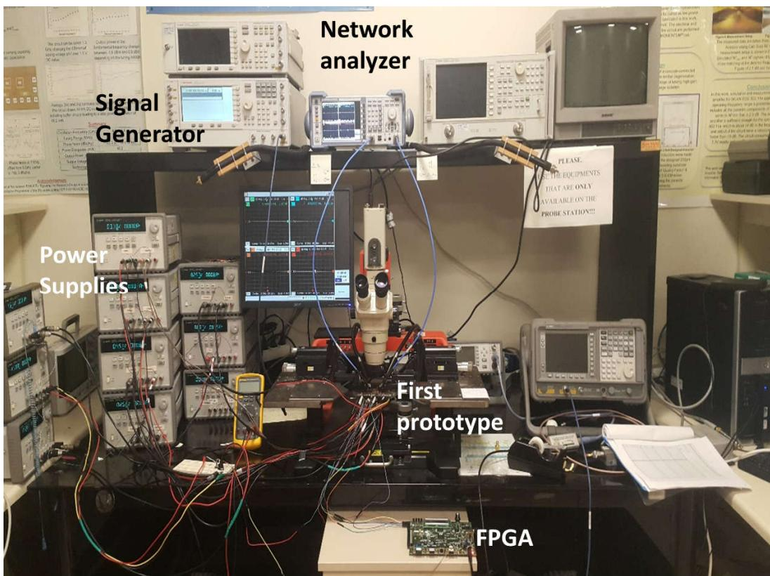
Fig. 53: Measurement Setup.
