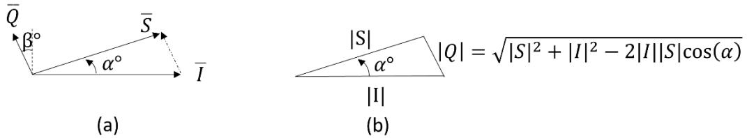
Fig. 12: a) Vector representation, b) Geometric approximation
