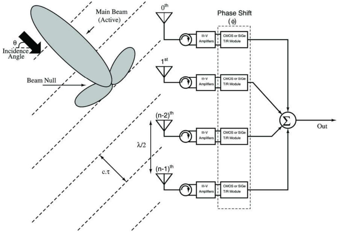
Fig. 1: Typical block diagram of the active electronically scanned phased-array radar system.
