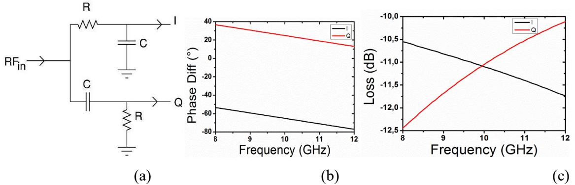
Fig. 7: a) RC-CR network b) phase difference c) S21 variation of I and Q.
