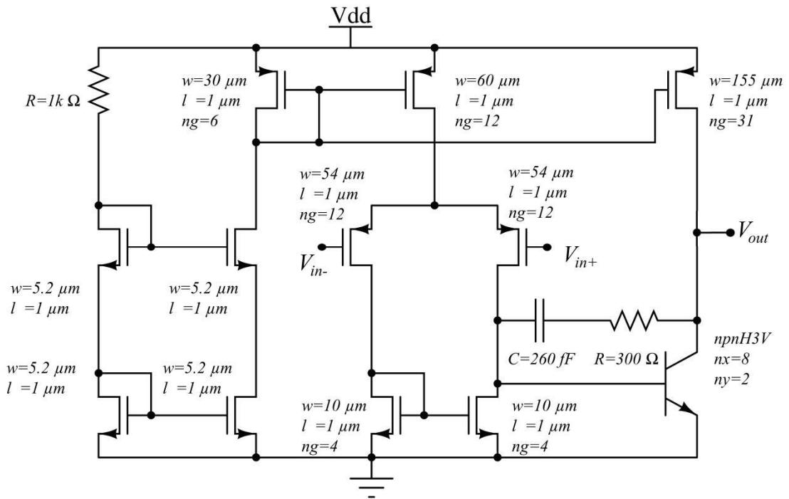
Fig. 32: OTA schematic with optimized transistor geometries.
