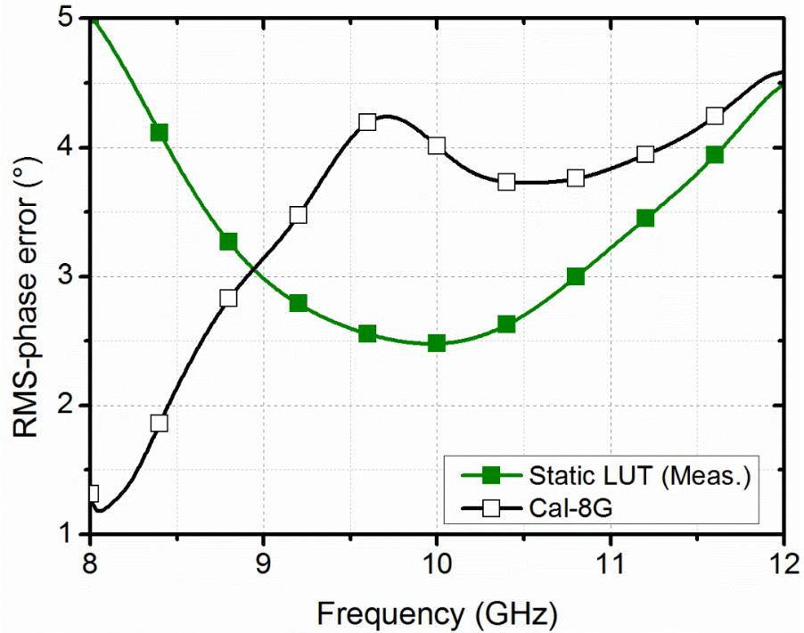
Fig. 59: The effect of I/Q phase-amplitude imbalance can be compensated through the recalibration at corner frequencies.
