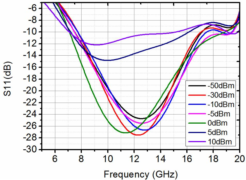
Fig. 27: S-parameter measurement results for 7 different input amplitudes.  $S_{11}$  is lower than -8 dB in 7-20 GHz and 52 dB dynamic range.
