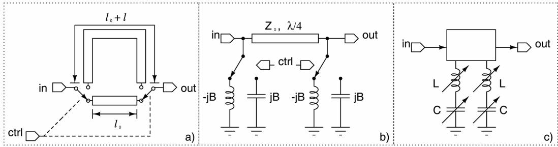
Fig. 3: a) Switched line phase shifter, b) Loaded line phase shifter, c) Reflection type phase shifter.
