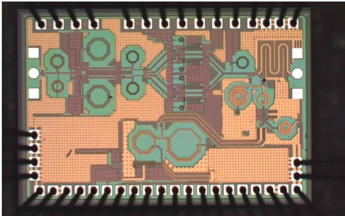
Fig. 51: Die photo of the first prototype consisting of Phase shifter, coupler, amplifier and power detector.
