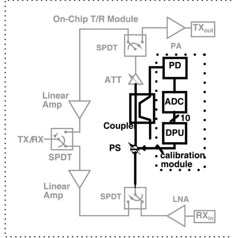
Fig. 14: Integration of the calibration module to T/R module.
