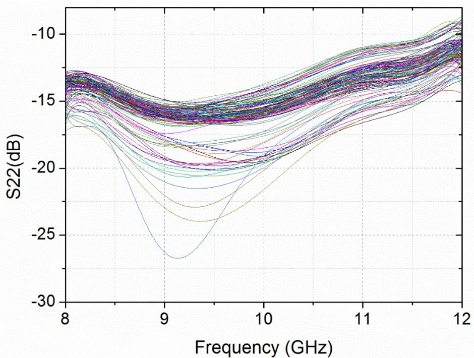
Fig. 62: Output return loss of proposed technique for 128 phase states.
