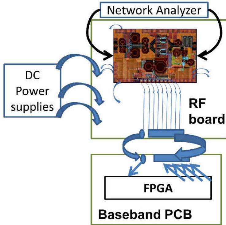
Fig. 52: Measurement plan of the first prototype.
