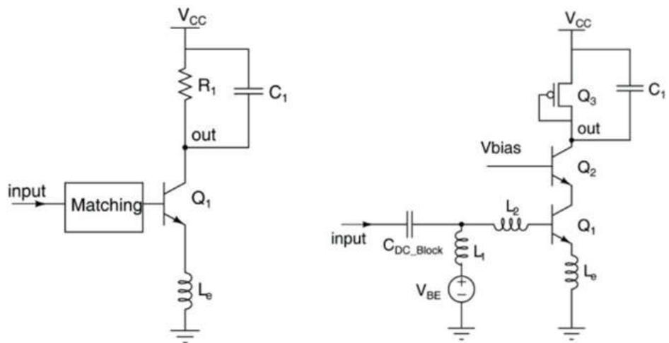
Fig. 22: (a) Conventional power detector. (b) Proposed power detector with increased input power dynamic range.
