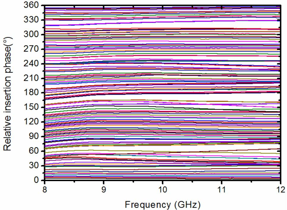
Fig. 55: Measured relative insertion phase response of PS after calibration.
