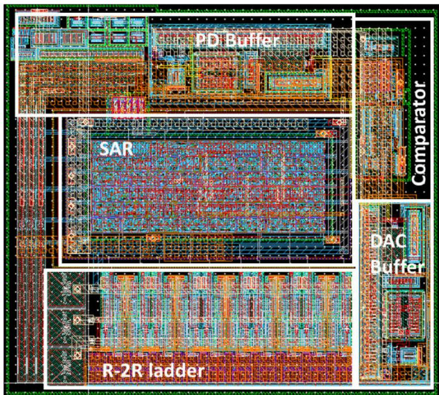
Fig. 35: Layout of the ADC.
