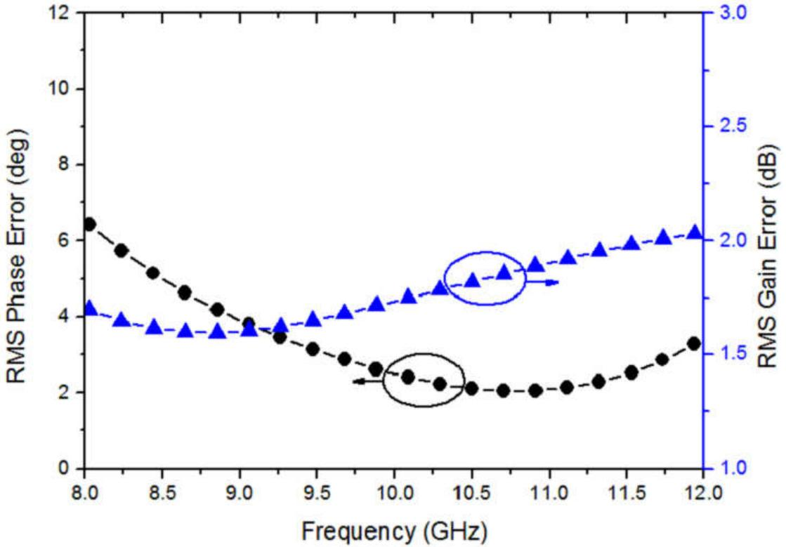
Fig. 21: Measured rms phase and gain error of previously fabricated vector sum based phase shifter with static LUT.
