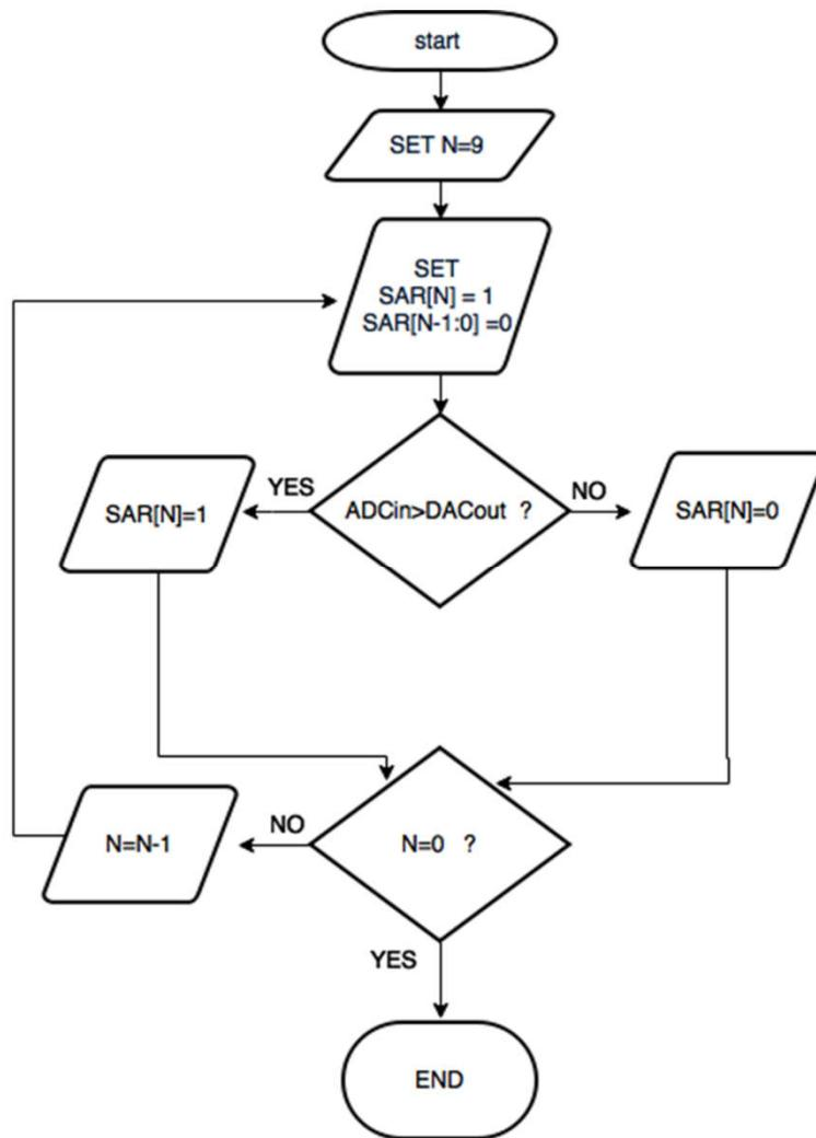
Fig. 31: Flowchart of the SAR algorithm.
