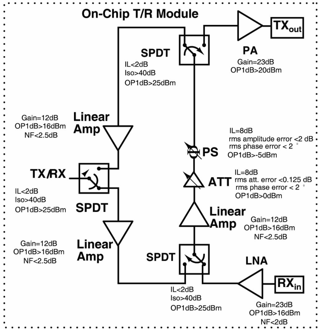
Fig. 2: Block diagram of proposed X-band phased-array transmit/receive core chip.
