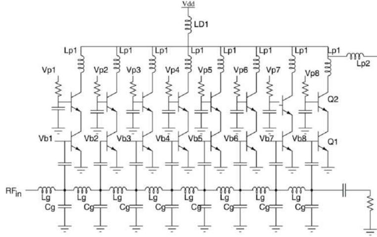
Fig. 5: 3-bit phase shifter using distributed active switches [47].
