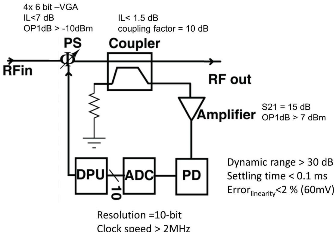
Fig. 17: Proposed system with block level specifications.
