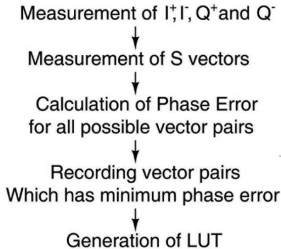
Fig. 15: Summary of proposed calibration algorithm.
