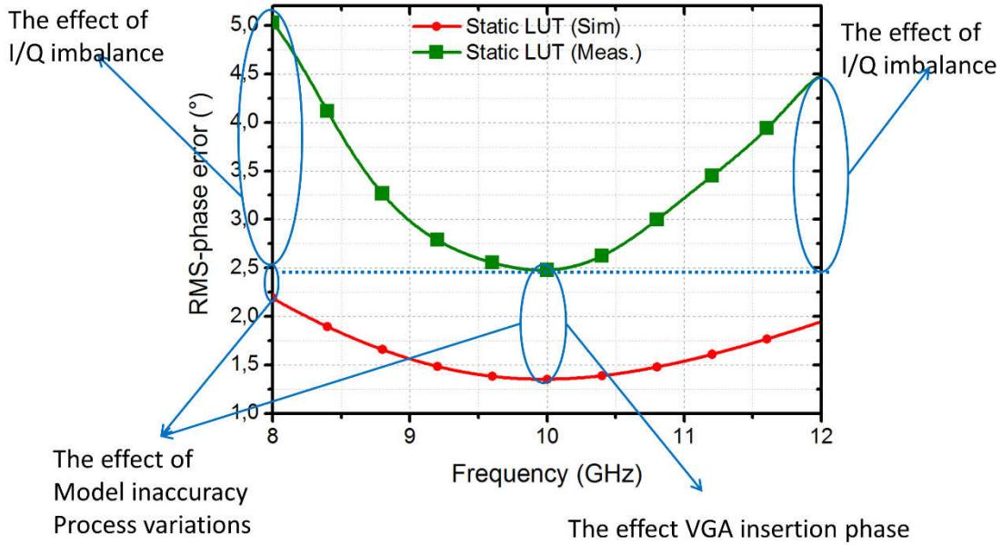
Fig. 56: Comparison of simulation and measurement results of phase shifter with *Static LUT* which is based on post layout simulation results.
