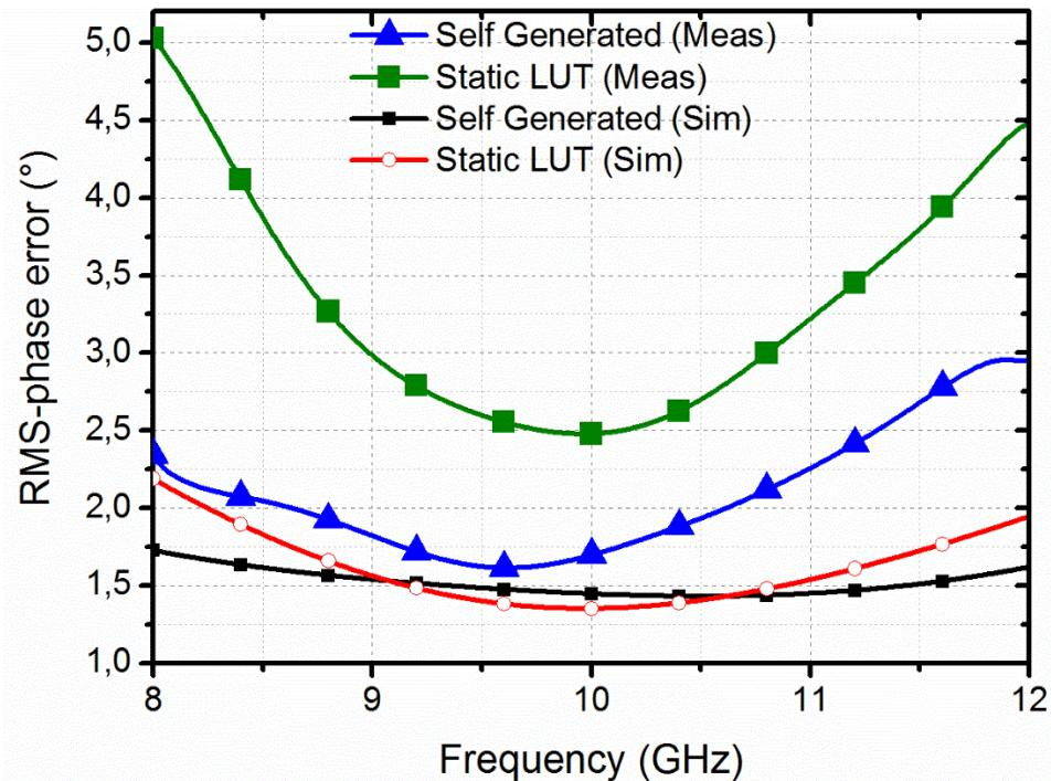
Fig. 57: Comparison of rms phase error simulations and measurement results of phase shifters. *Static LUT* curves represent the results of the phase shifter with a LUT which is based on post layout simulation results. *Self-Generated* curves represent results of the proposed technique.
