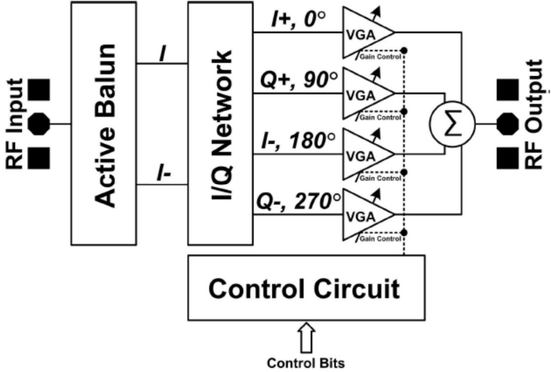
Fig. 6: Block diagram of vector sum type phase shifter.
