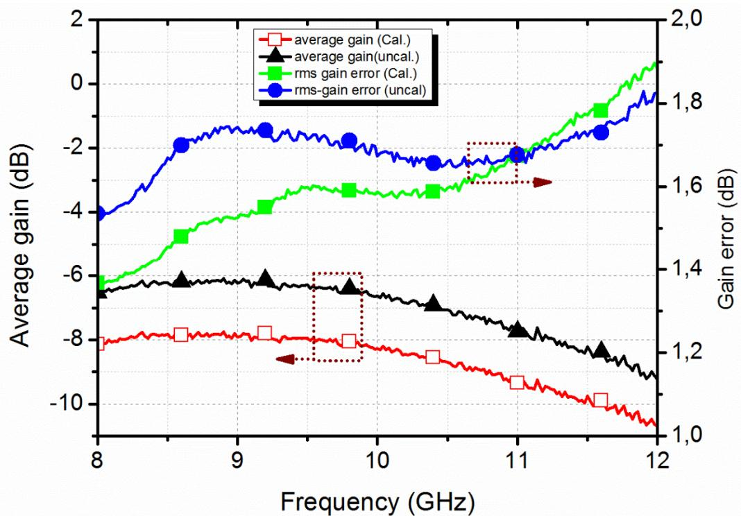
Fig. 61: Average gain and rms gain error measurements of phase shifter.
