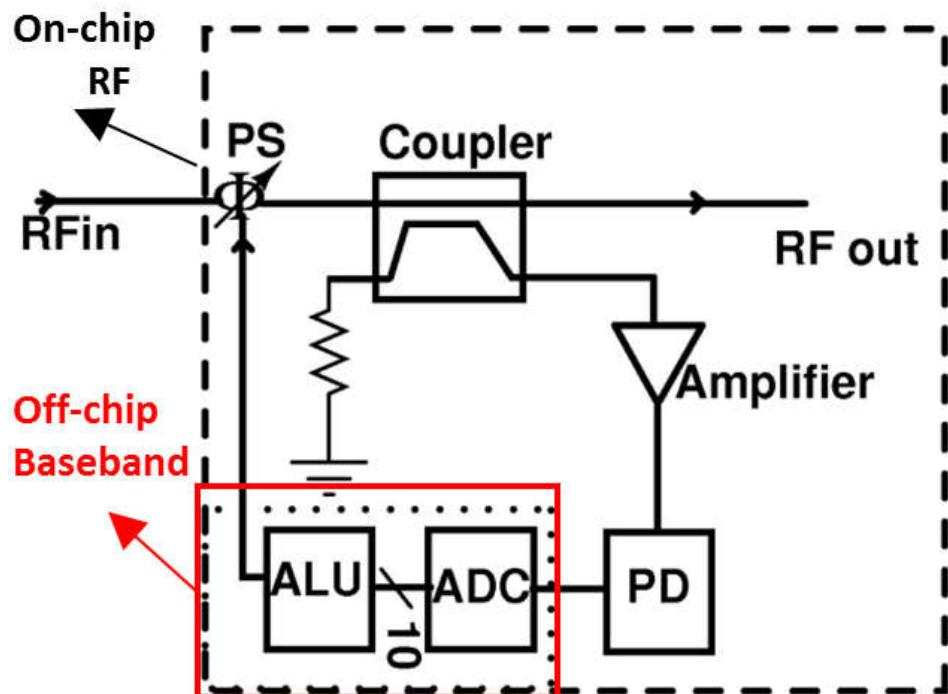
Fig. 37: On-Chip RF circuits and PD are combined in the first prototype. For baseband circuits, off-chip components will be used.
