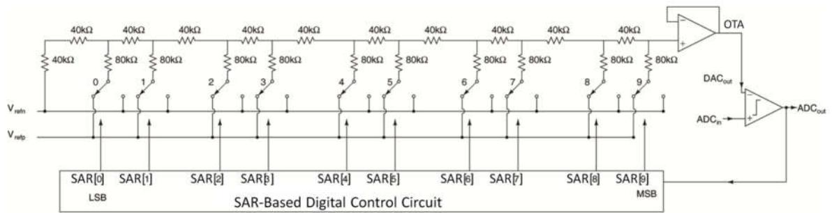
Fig. 30: Block diagram of SAR based ADC.
