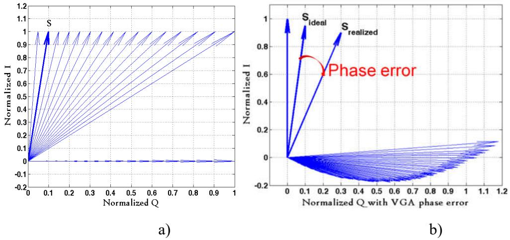
Fig. 11: a) Vector sum with ideal vectors, b) Vector sum including VGA phase error. VGA phase error in this figure is imported from post layout simulations.
