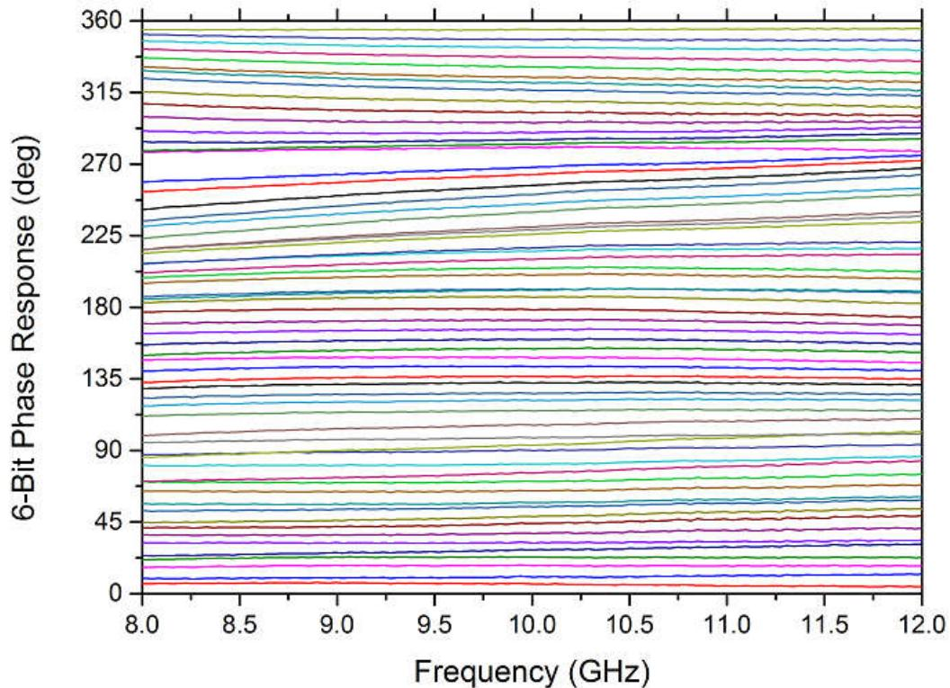
Fig. 20: Measured Relative insertion phase response of previously fabricated vector sum based phase shifter with static LUT.
