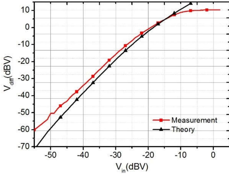
Fig. 26: Logarithmic-Logarithmic plot of output DC voltage change vs input signal amplitude.
