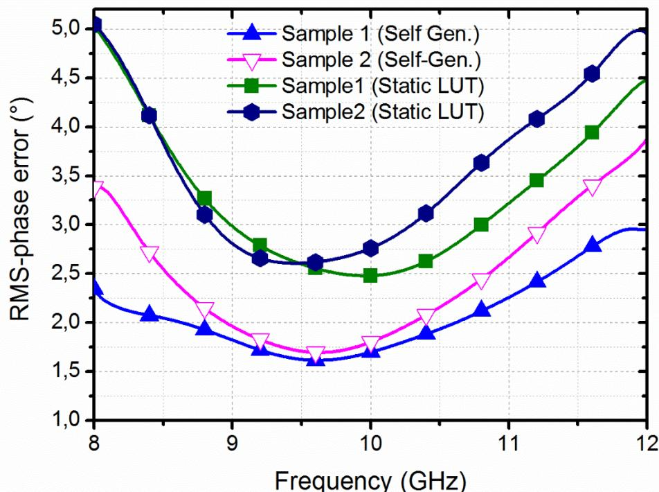
Fig. 58: rms phase error measurement results for different dies.
