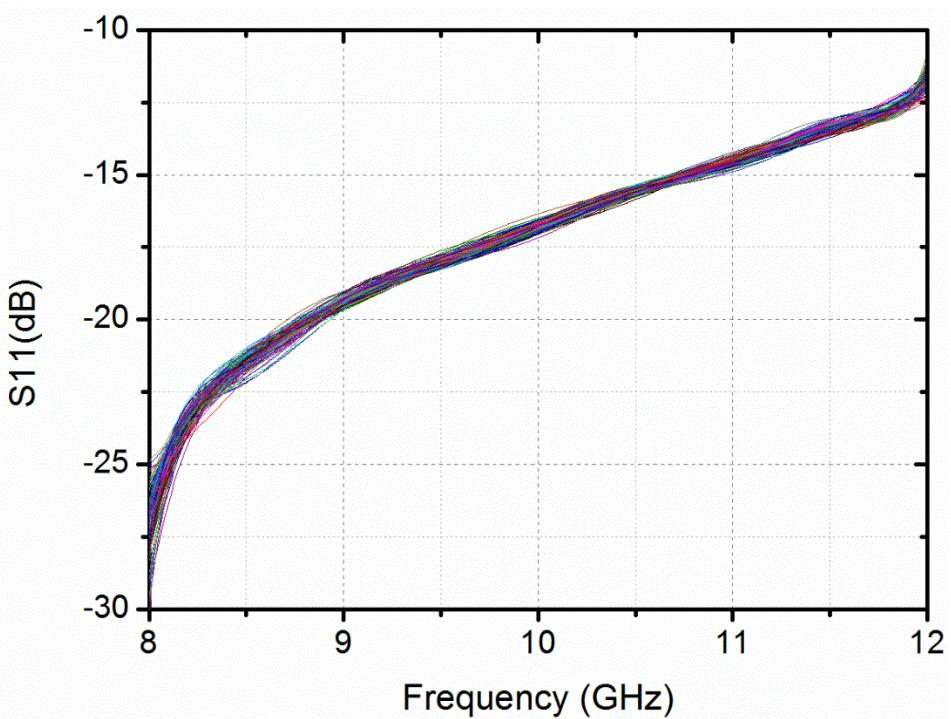
Fig. 63: Input return loss of the proposed technique for 128 phase states.
