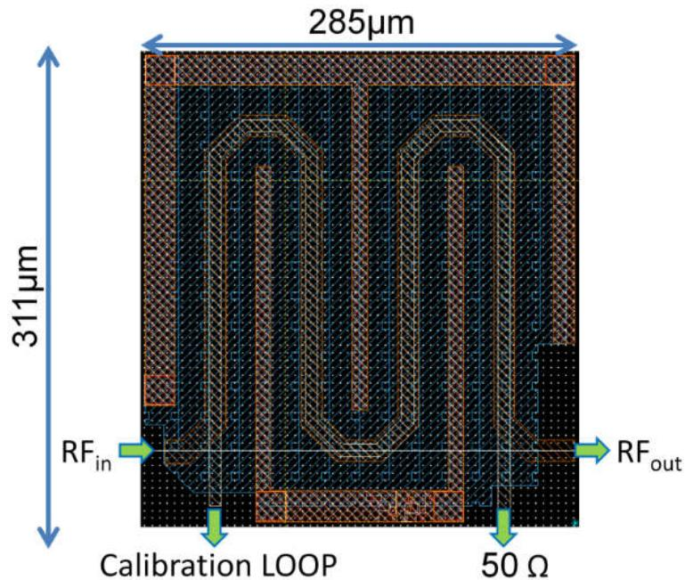
Fig. 28: Layout of the coupler, width of the top M2 is 14  $\mu\text{m}$ , width of the top M1 is 8  $\mu\text{m}$ , length is 960  $\mu\text{m}$ .
