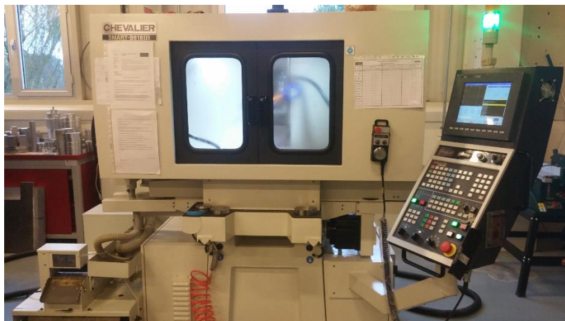
Figure 51: CNC grinding machine
