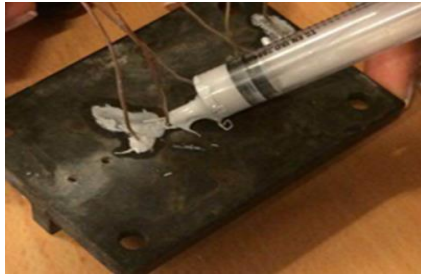
Figure 55: Thermocouple fixation with syringe
