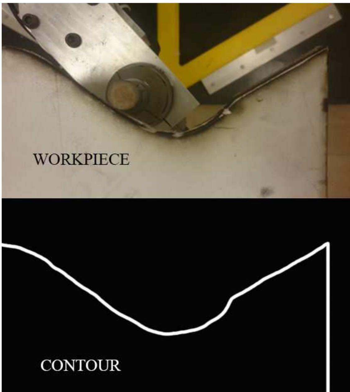
*Figure 1.1: Sample of the contour of the workpiece used in the experiments*
