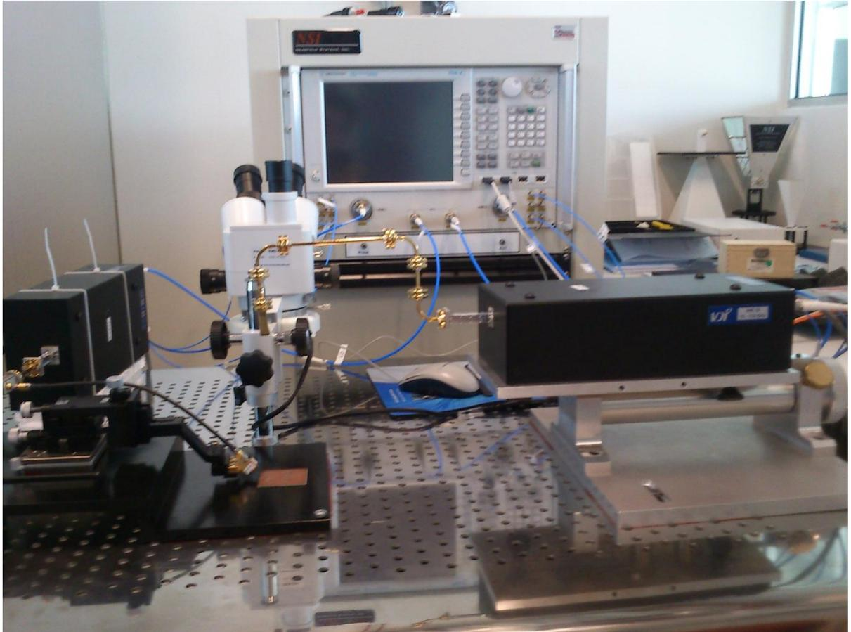
Fig. 4.2 Implemented Millimeter Wave Antenna Setup
