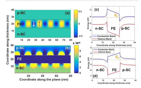
**Figure 4.** (a) Polarization map, (b) free electron density, (c) hole density, (d) flat band structure showing the band bending along the thickness along a +sign domain and (e) a -sign domain for the nSC/FE/pSC stack with  $10^{20}$  cm<sup>-3</sup> donor density in the nSC and  $10^{17}$  cm<sup>-3</sup> acceptor density in the pSC at 0V top electrode bias. The dashed horizontal lines in (c,d) indicate the Fermi level of the stack (E<sub>F</sub>) computed from Eqs 5-10.
