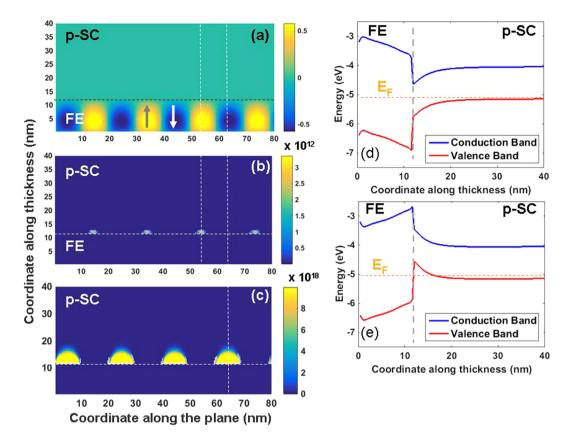
**Figure 2.** (a) Polarization map, (b) free electron density, (c) hole density, (d) flat band structure showing the band bending along the thickness in a -sign domain and (e) along a + sign domain for the m/FE/pSC stack with  $10^{17}$  cm<sup>-3</sup> acceptor density in the pSC at zero bias. Note that in (b) free electrons are highly confined. The dashed horizontal line in (d,e) indicate the Fermi level of the stack (E<sub>F</sub>) computed from Eqs 5–10.
