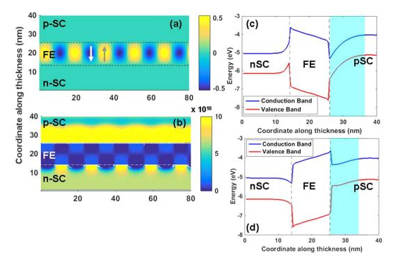
**Figure 5.** (a) Polarization map, (b) free electron density, (c) flat band structure showing the band bending along the thickness in a +sign domain and (d) along a -sign domain for the nSC/FE/pSC stack with  $10^{20}$  cm<sup>-3</sup> donor density in the nSC and  $10^{17}$  cm<sup>-3</sup> acceptor density in the pSC at 1 V bottom electrode bias. Note the band bending favoring free electron accumulation at the FE/pSC interface of the -sign domain in the MD state under bias.
