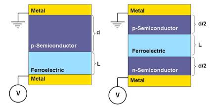
Figure 1. Schematics of the two thin film stacks studied in this work (a) m/FE/pSC and (b) nSC/FE/pSC, both systems with ideal electrodes.
