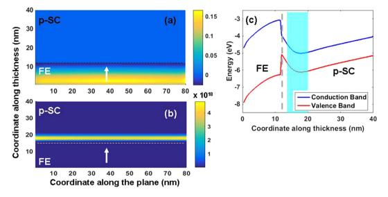
**Figure 3.** (a) Polarization map, (b) free electron density, (c) flat band structure showing the band bending along the thickness in a +sign domain for the m/FE/pSC stack with  $10^{17}$  cm<sup>-3</sup> acceptor density in the pSC at 1.5 V bottom electrode bias. The shaded region in (c) indicates the electron accumulation at the FE/pSC interface.
