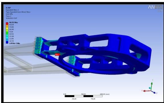
**Figure 7: Maximum stress on cast nacelle part. (1)**
