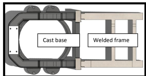
Figure 1 :Top view of hybrid bedplate design. (1)
