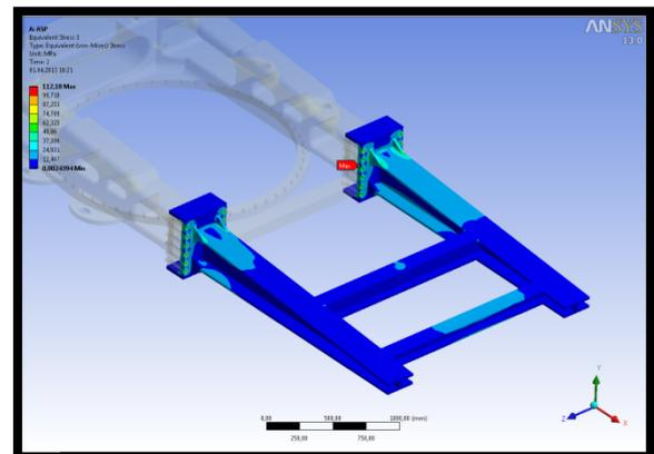
**Figure 9: Minimum stress on welded frame.**
