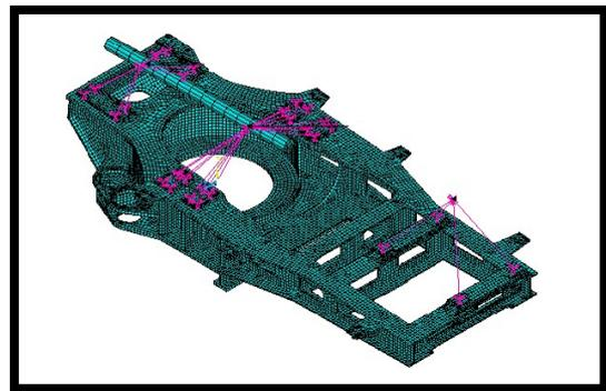
Figure 3: Meshed model of a sample bedplate. (4)
