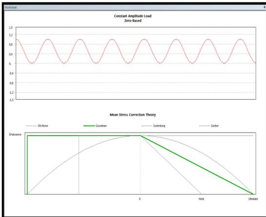
Figure 2: Zero based stress cycles. (2)
