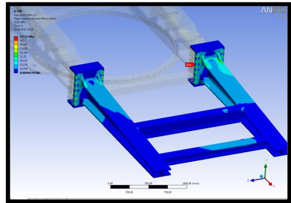
**Figure 8 : Maximum stress on welded profile part.**
