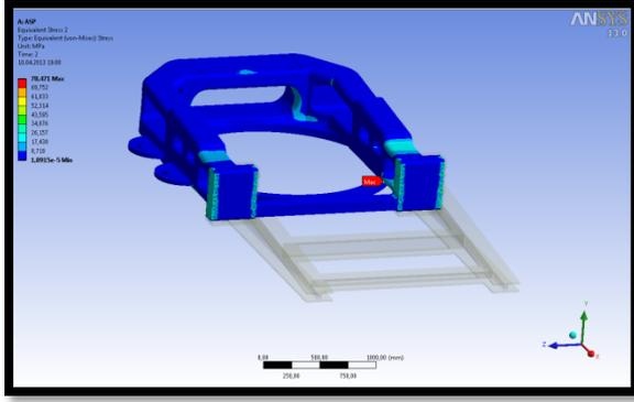
Figure 10 : Minimum stress on cast part. (1)
