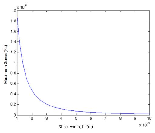
Figure 4.18- Maximum stress vs actuator width (Other parameters are kept constant).
