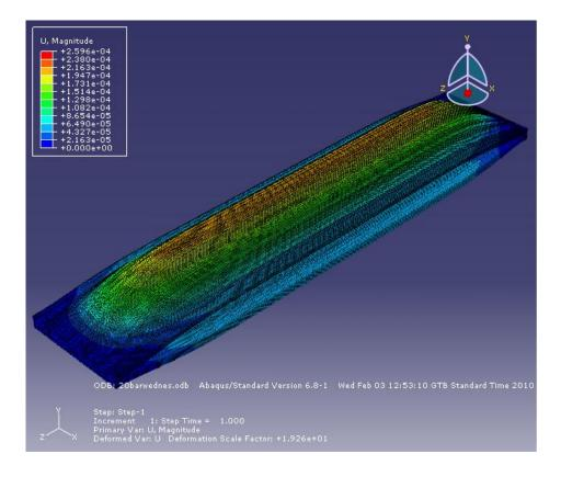
Figure 4.31– FEA displacement results for 20 bar interior pressure.
