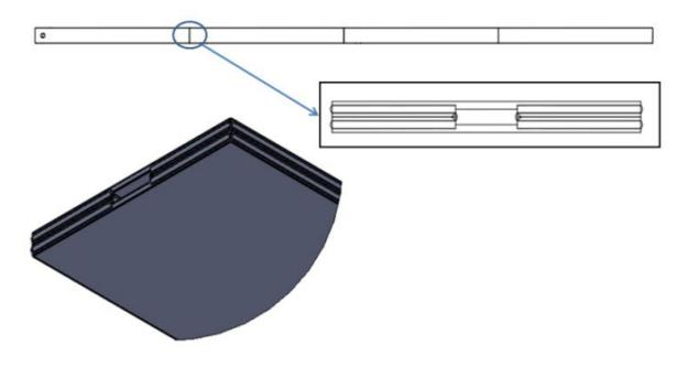
Figure 4.24- Seam welding locations between the cells.
