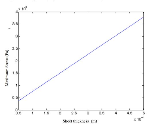
Figure 4.16 – Maximum stress vs sheet thickness. (Other parameters are kept constant)
