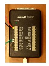
Figure 3.10 – miniLAB 1008 10 bit data acquisition card.
