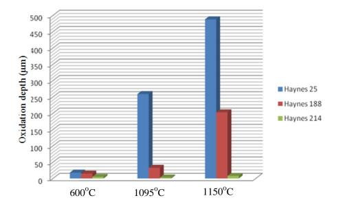
Figure 4.4 – Oxidation depth of candidate materials at elevated temperatures.
