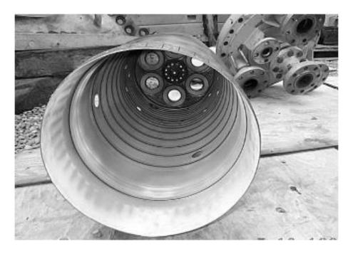
Figure 1.4 – Combustion can [4]
