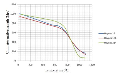
Figure 4.2 – Tensile strength of candidate materials at elevated temperatures
