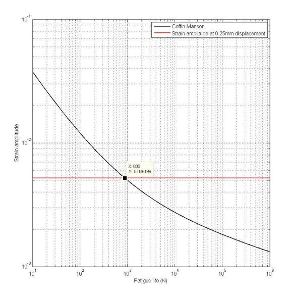
Figure 4.34 – Low cycle fatigue life curve for actuator Design B
