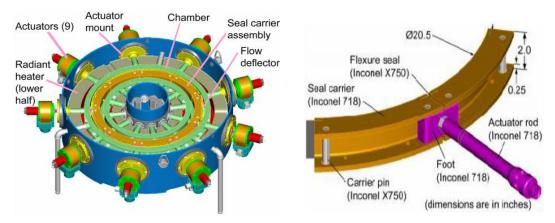
Figure 2.1 – NASA's first generation ACC test rig.
