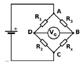
Figure 3.7- Wheatstone bridge circuit diagram
