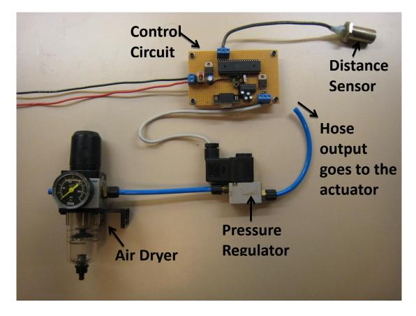
Figure 5.5 – Electronic Control System
