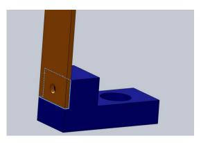
Figure 5.8- Actuator is connected to the test rig and fixed by the connector shown in blue.
