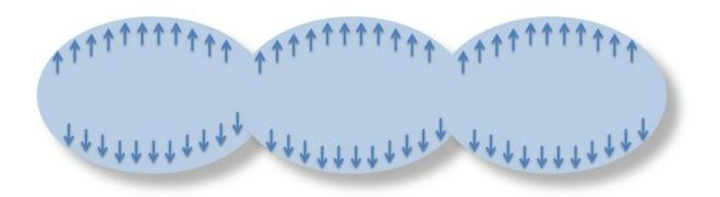
Figure 4.6- Cross section of the pressurized actuator
