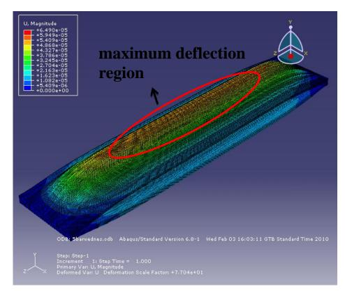
Figure 3.27 – FEA displacement results for 5 bar interior pressure
