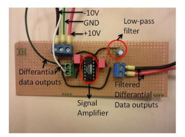
Figure 3.8 - Amplifier and low-pass filter circuit
