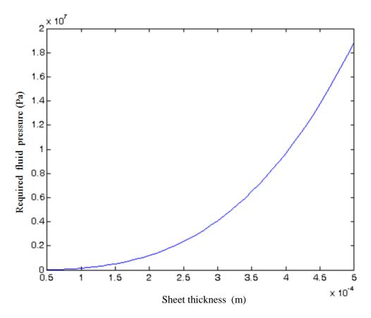
Figure 4.15- Required liquid pressure to achieve 0.25mm displacement vs sheet thickness
