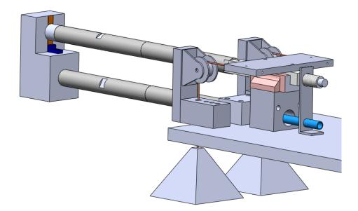
Figure 5.2- Isometric view of the actuator test rig
