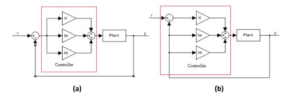
**Figure 5.4** (a) PID controller with error feedback
