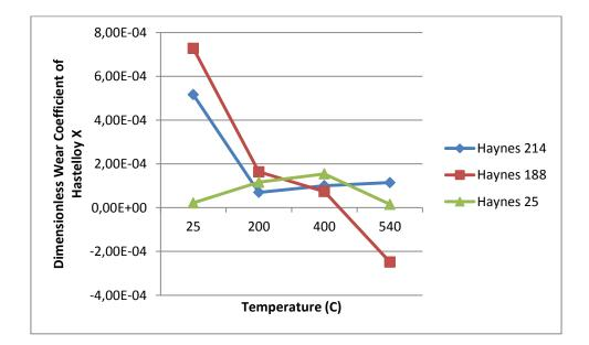
Figure 3.14– Dimensionless wear coefficients of Hastelloy X pins against H25, H188 and H214 sheets.
