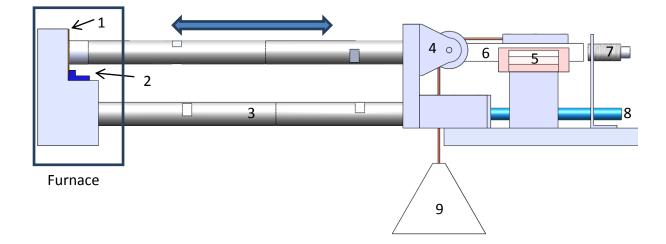
**Figure 5.1** Actuator test rig consists of; high temperature actuator (1), actuator connector (2), rods (3), two pulleys (4), linear slide – car (5), linear slide – rail (6), displacement sensor (7), air inlet (8) and dead weight (9)
