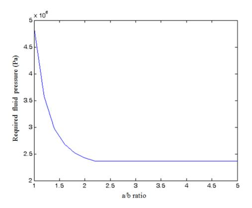
Figure 4.13 – Required liquid pressure in order to achieve 0.25 mm displacement vs a/b ratio
