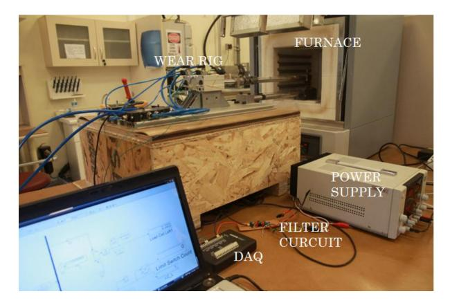
Figure 3.2- Complete picture of the wear rig
