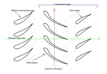
Figure 1-2- Axial flow compressor rotor blades and stator vanes
