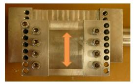
**Figure 3.5** – Lower specimen holder can slide to achive multiple wear tracks from single specimen.
