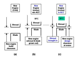
Figure 1.7 - Blade tip clearance control concept
