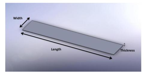
Figure 4.9 - Dimensions of selected actuator cell for Design A: Length=50mm, Width=10mm, Thickness=0.25mm
