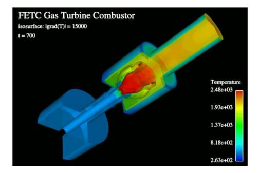
Figure 1.3 – A combustor model
