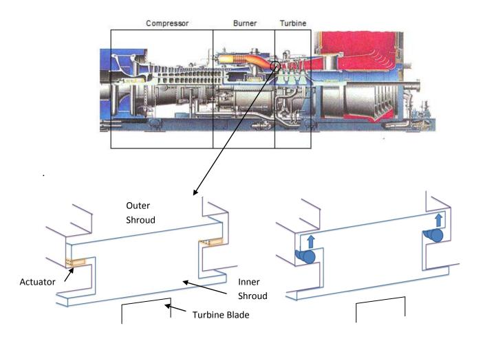
Figure 4.7 – Actuator position in the gas turbine.
