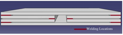
Figure 5.7 – Welding locations of the actuator
