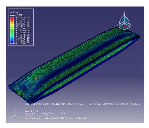
Figure 4.30 – FEA stress results for 10 bar interior pressure.
