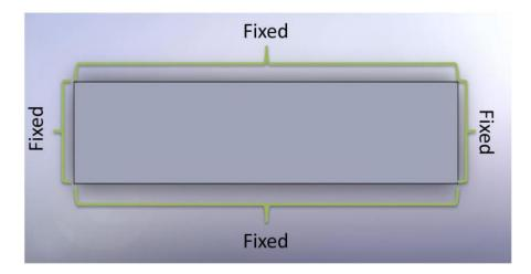
Figure 4.10 – Boundary conditions of the actuator
