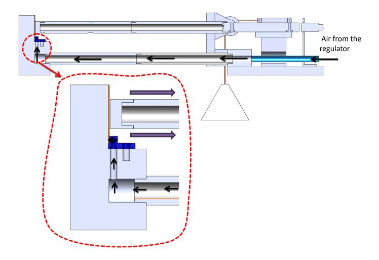
Figure 5.3 – Pressurized air's path from the pressure regulator to the actuator.
