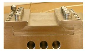
**Figure 3.4** – Three components of the lower speciment holder.
