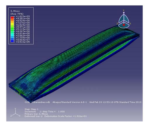
Figure 4.32– FEA stress results for 20 bar interior pressure
