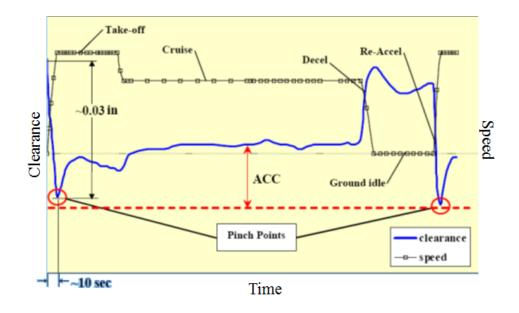
Figure 1.6 - Clearance variation during operating cycle of a jet engine
