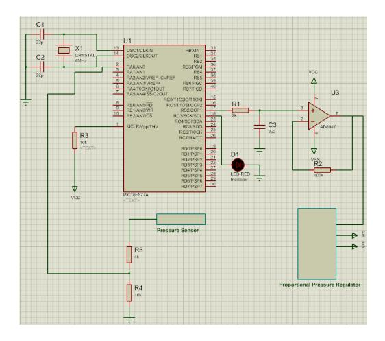
Figure 5.6 - Schematic design of the control circuit
