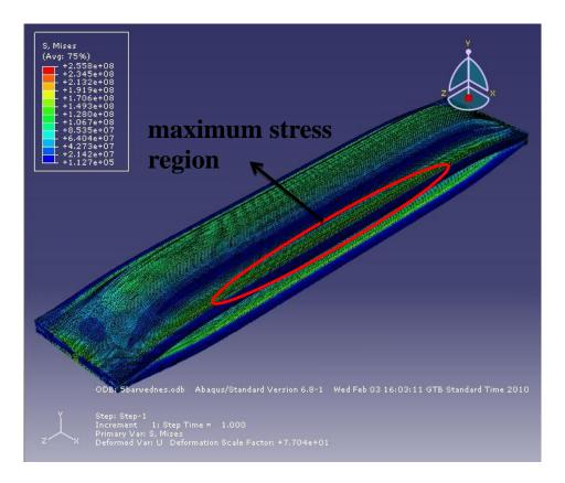
Figure 4.28 – FEA stress results for 5 bar interior pressure
