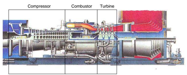
Figure 1-1 – Industrial gas turbine stages: compressor, combustor and turbine.
