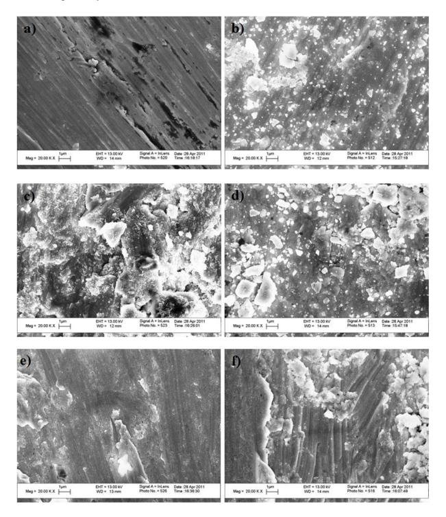
**Figure 3.15** – SEM photomicrographs showing portions of wear tracks with 20K magnification for a) Haynes 25, 400°C b) Haynes 25, 540°C) Haynes 188, 400°C d) Haynes 188, 540°C e) Haynes 214, 400°C f) Haynes 214, 540°C.
