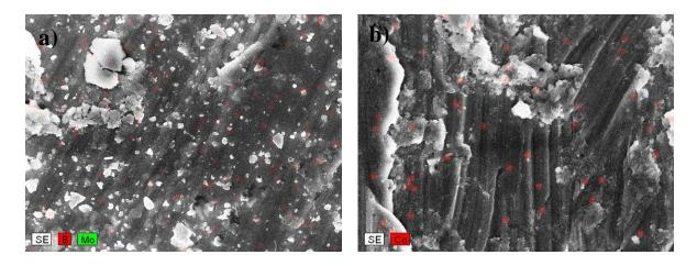
**Figure 3.17** a) Haynes 25 (Locations of transferred Boron from pin to sheet are marked in red.) b) EDX image of Haynes 214 (Locations of transferred Cobalt from pin to sheet are marked in red.)
