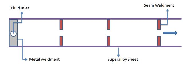
Figure 4.5 - Top view of the actuator.
