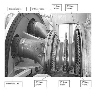
Figure 1.5 – Turbine stage
