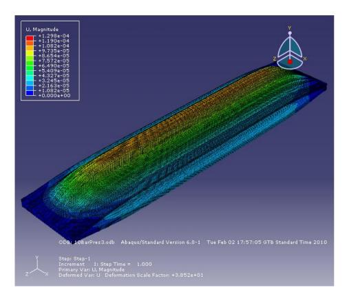
Figure 4.29 – FEA displacement results for 10 bar interior pressure.
