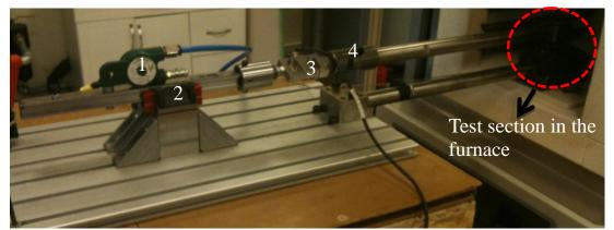
Figure 3.11 - Fretting wear rig is composed of pneumatic vibrator (1), linear slide (2), load cell (3), hinge (4).
