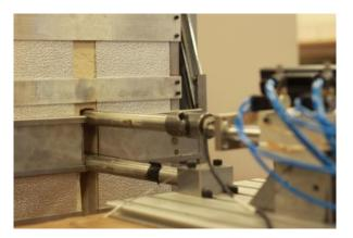
Figure 3.6- Test section is positioned in the furnace through access hole in the cover
