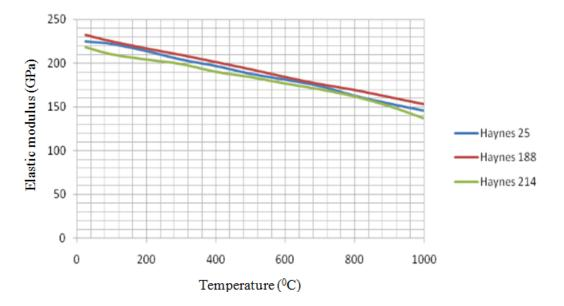
Figure 4.1 – Variation of elastic modulus of candidate materials with temperature.
