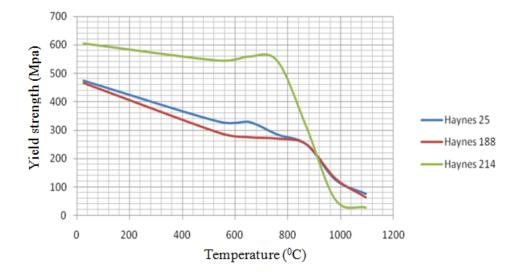
Figure 4.3 – Variation of yield strength for the candidate materials at elevated temperatures
