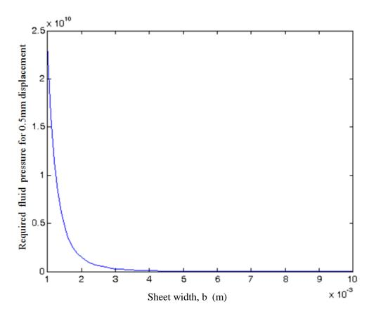
Figure 4.17 – Required liquid pressure to achieve 0.25mm displacement vs actuator width
