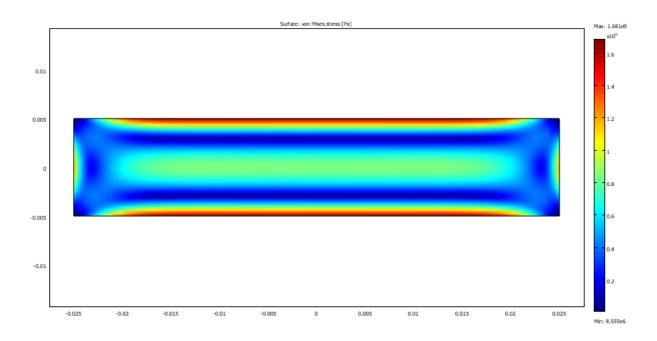
Figure 4.20– Stress distribution over the plate
