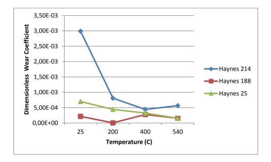
Figure 3.13– Dimensionless wear coefficients of H25, H188 and H214 sheets against Hastelloy X pin.
