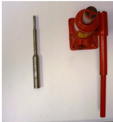
FIGURE 3.8: Hydraulic jack and cylindrical metal piece used for removal of the 3D specimen from the mold
