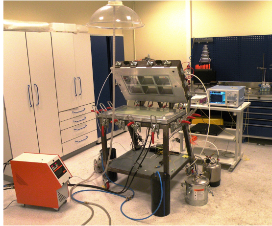
FIGURE 3.2: Inhouse built RTM system
