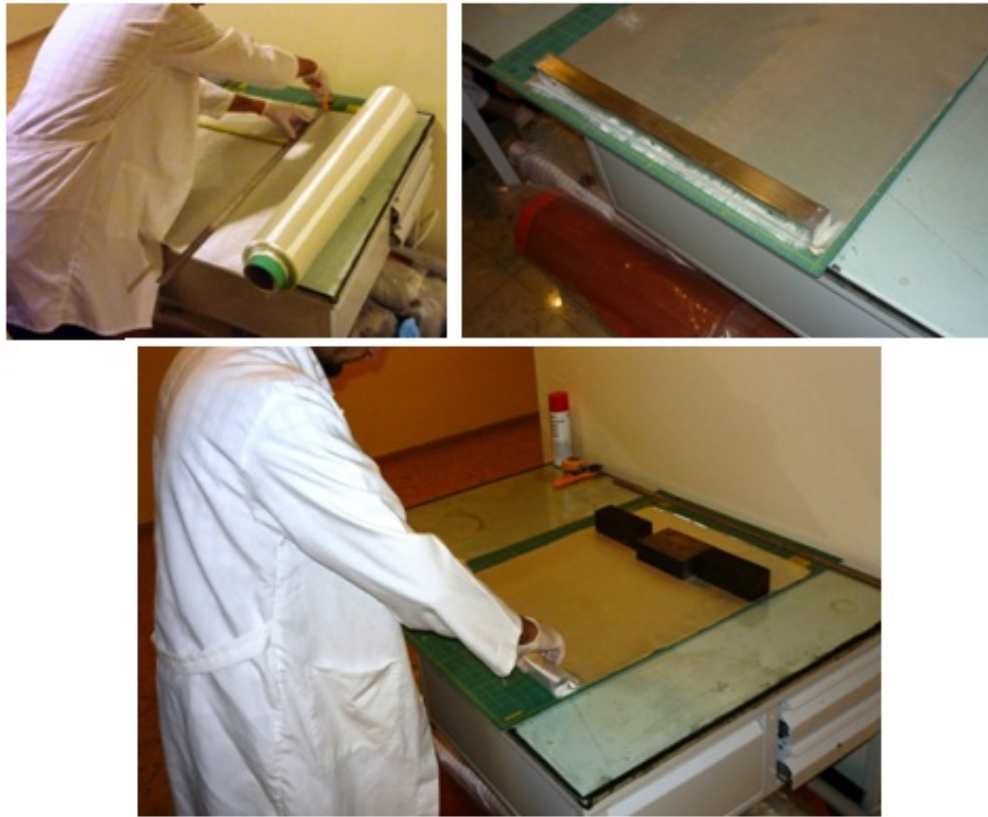
FIGURE 3.7: Wrapping the fabric around the square mandrel
