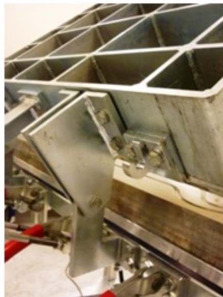
FIGURE 3.6: Hinge that connects the lid and the mold
