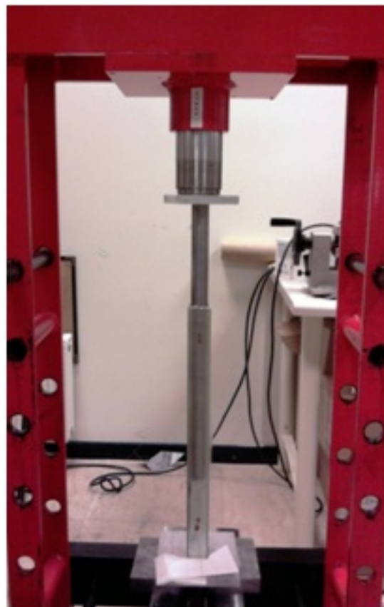
FIGURE 3.10: The process of removal of the mandrel with hydraulic press
