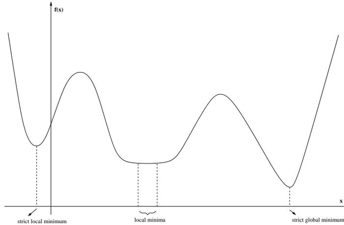
Figure 1.1: Local and global minimizers of a single dimensional problem [7]
