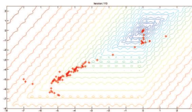
(b) Iteration 113: Complete path of individual TR with BFGS
