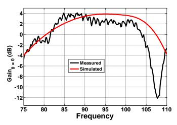
Fig. 9. Measured and simulated antenna gain versus frequency.
