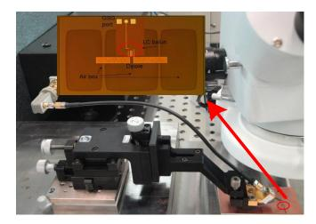
Fig. 5. Manufactured antenna and measurement setup.
