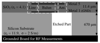
Fig. 2. Cross section view of the etched substrate and different layers illustration.
