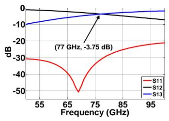
Fig. 3. Simulated reflection coefficient at P1 (S11) and scattering parameters between P1-P2 (S12) and P1-P3 (S13) ports.
