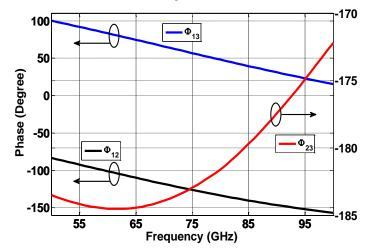
Fig. 4. Left-side scaling for simulated phase difference between P1-P2 ( $\Phi_{12}$ ), P1-P3 ( $\Phi_{13}$ ) and right-side scaling for P2-P3 ( $\Phi_{23}$ ) ports.
