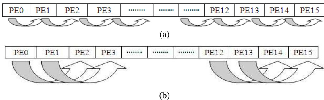
Figure 4.6 Shifting in PE array (a) 1 pixel, (b) 2 pixels
