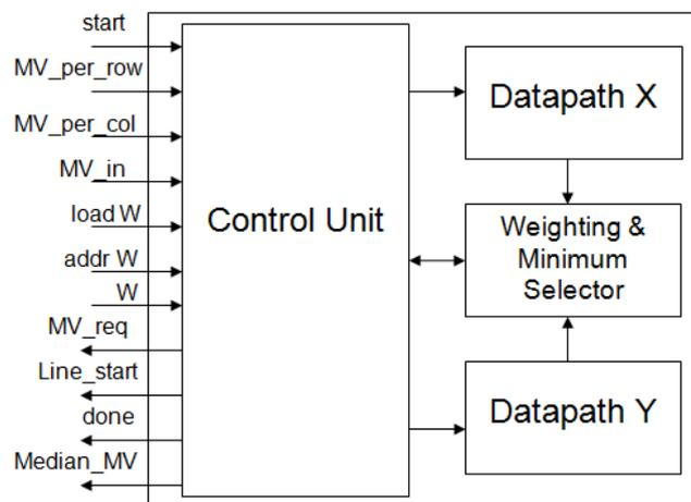
Figure 5.7 Top-level block diagram of the VMF hardware
