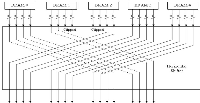
Figure 3.17 Ten byte rotate left operation done by the horizontal shifter
