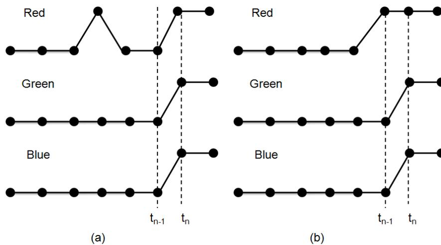
Figure 5.4 M-Ordering based VMF (a) input, (b) output
