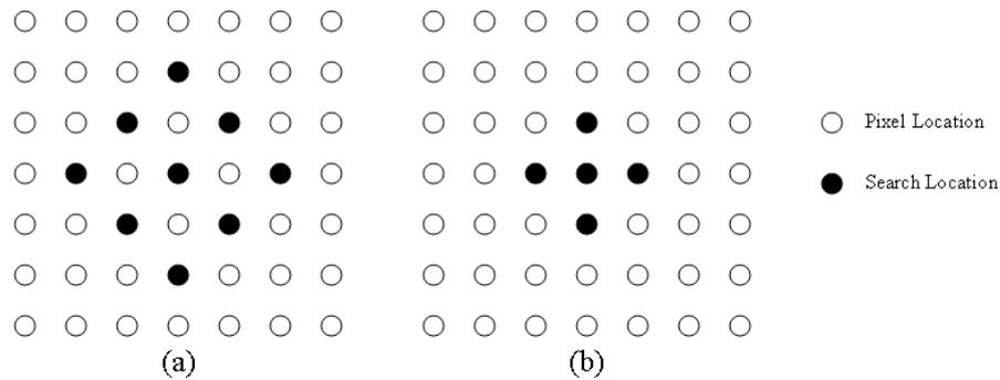
Figure 2.10 The DS algorithm (a) LDSP, (b) SDSP
