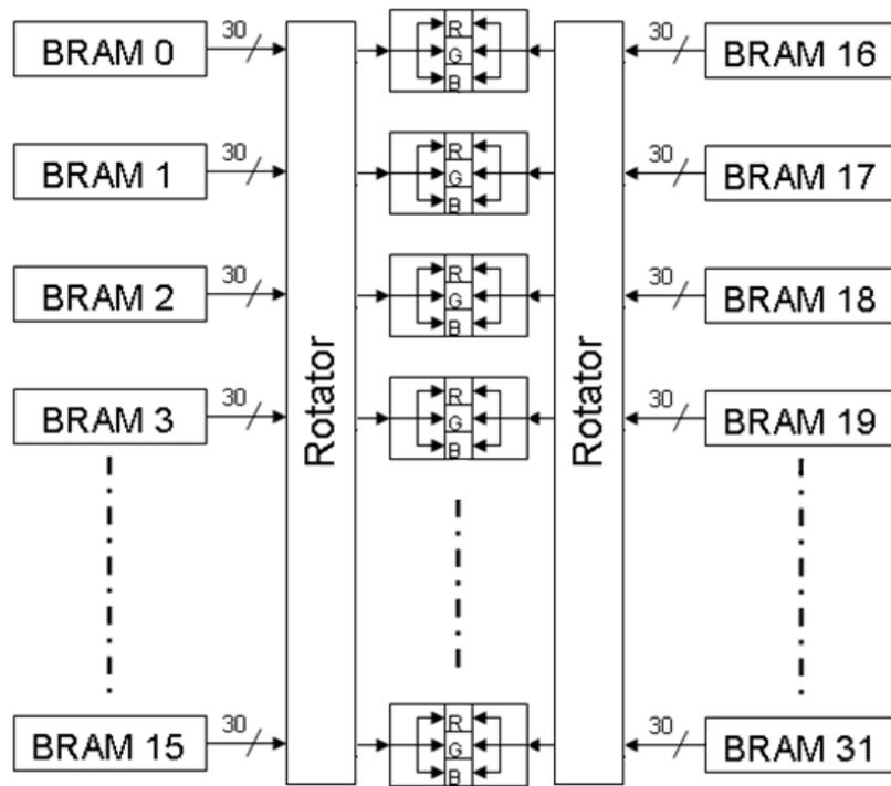
Figure 6.9 On-chip memory and datapath
