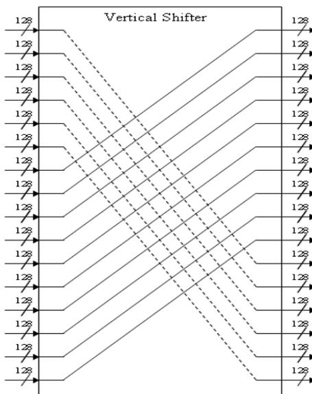
Figure 3.18 Six line rotate left operation done by the vertical shifter
