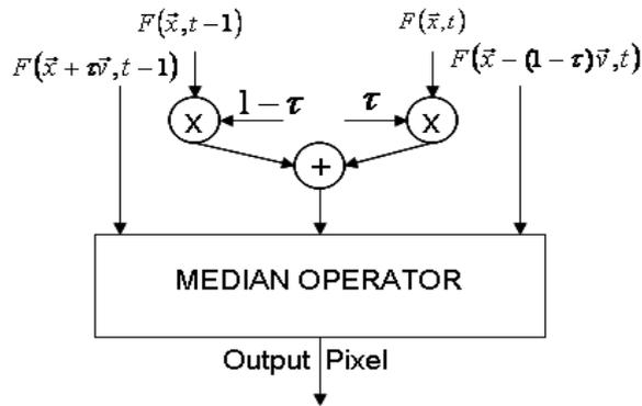
Figure 6.4 The block diagram of DMF
