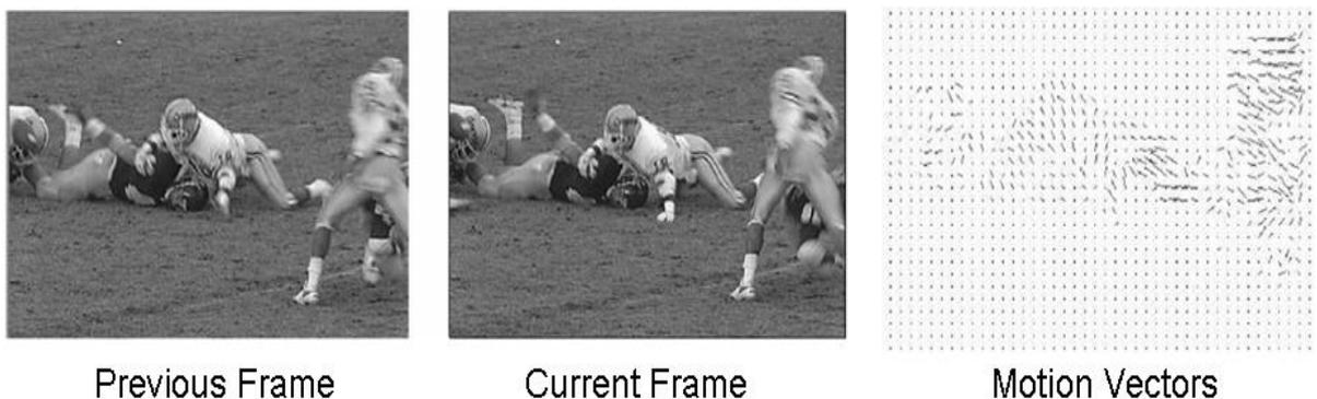
Figure 2.2 A BM ME example and the resulting MVF
