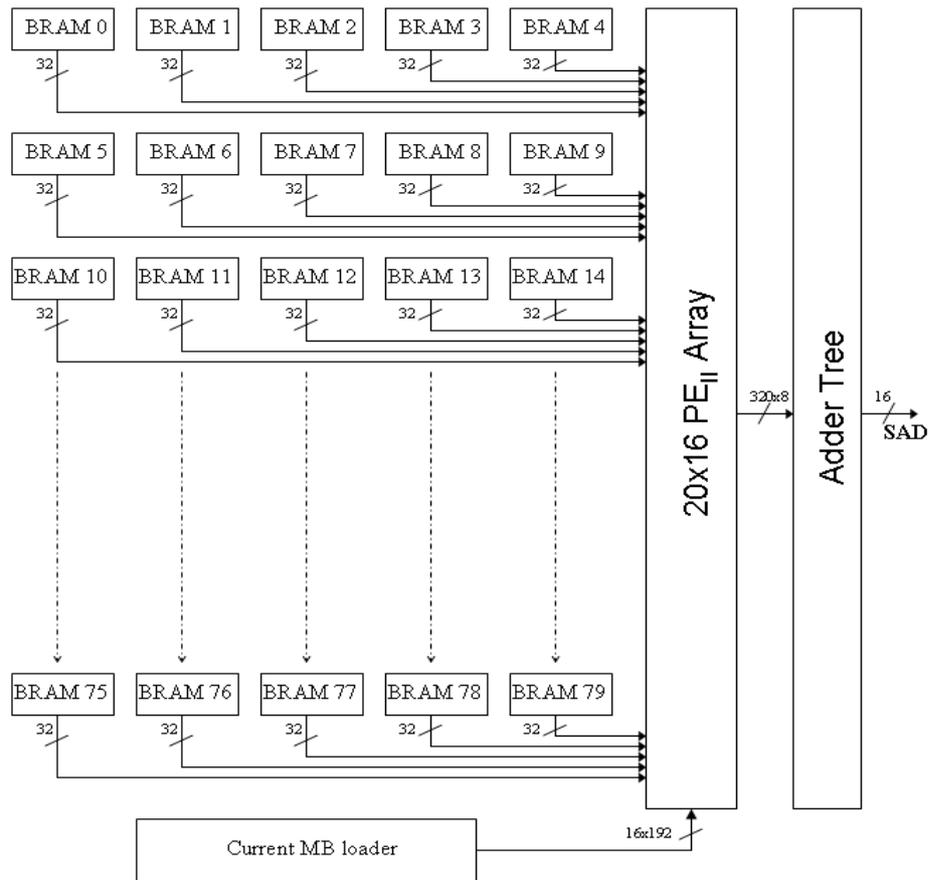
Figure 3.11 Block diagram of the implementation type II
