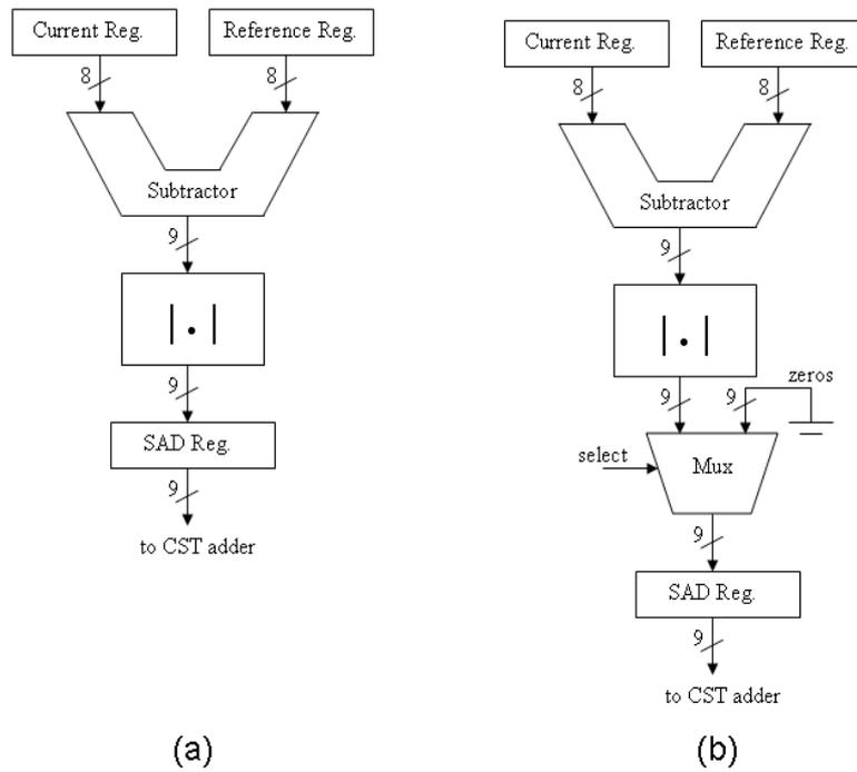
Figure 3.9 Block diagram of processing elements: (a) PE<sub>I</sub>, (b) PE<sub>II</sub>
