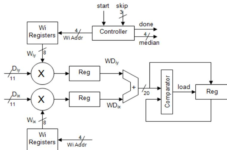
Figure 5.9 Block diagram of the weighting and minimum selector module
