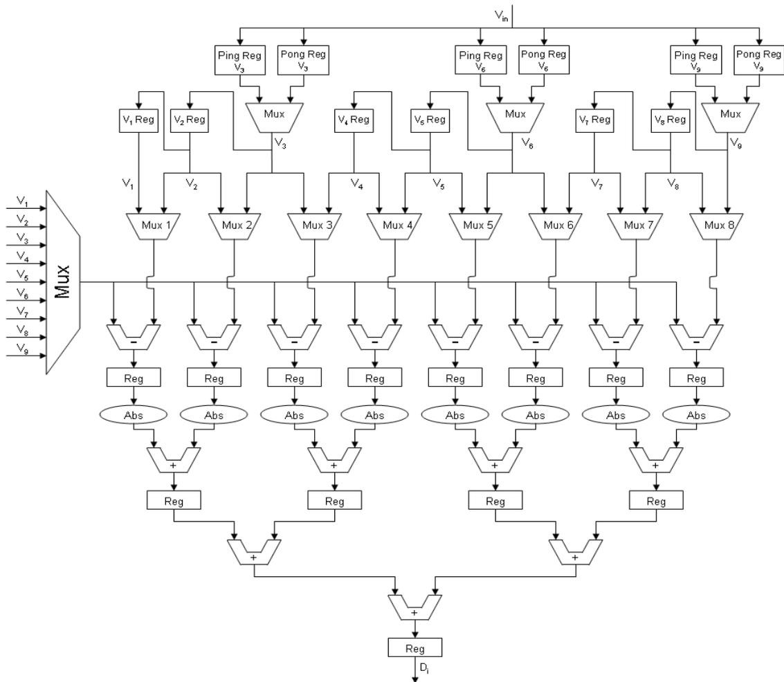
Figure 5.8 Block diagram of the VMF datapath
