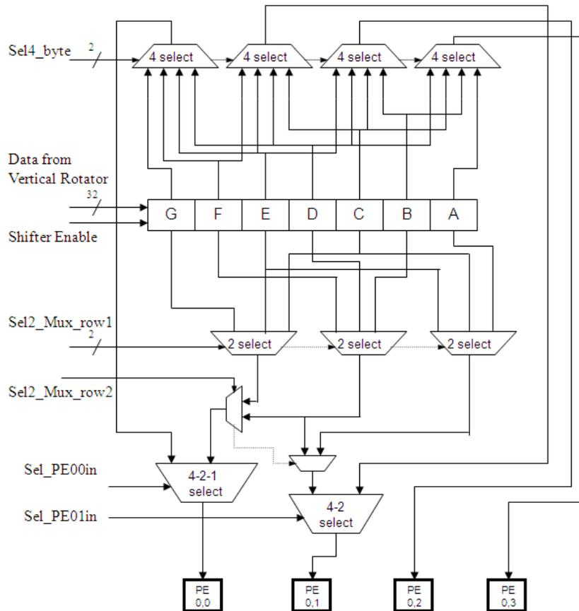
Figure 4.8 Multiplexing unit
