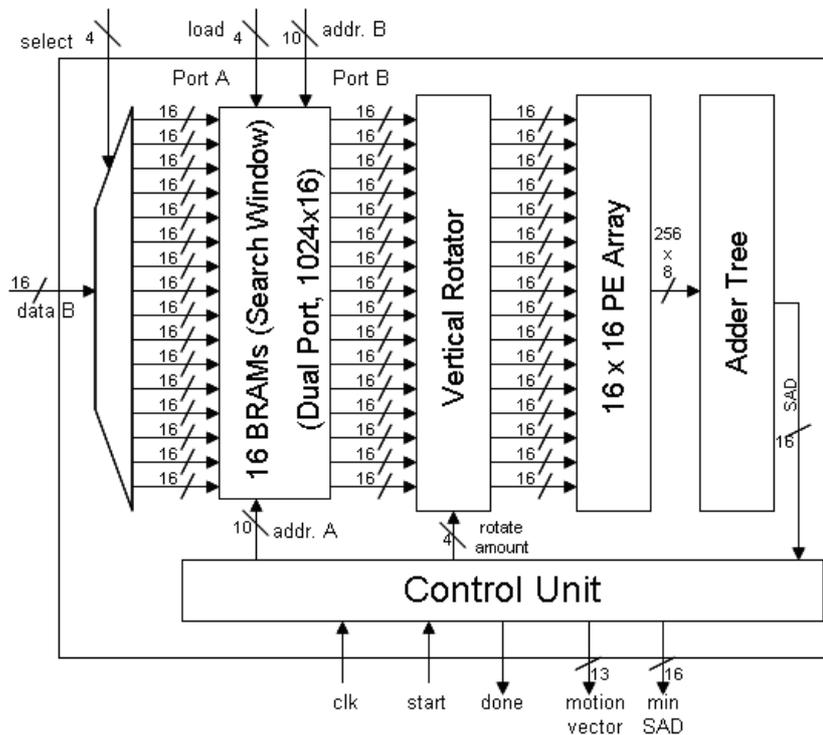
Figure 3.19 Top-level block diagram of the systolic architecture
