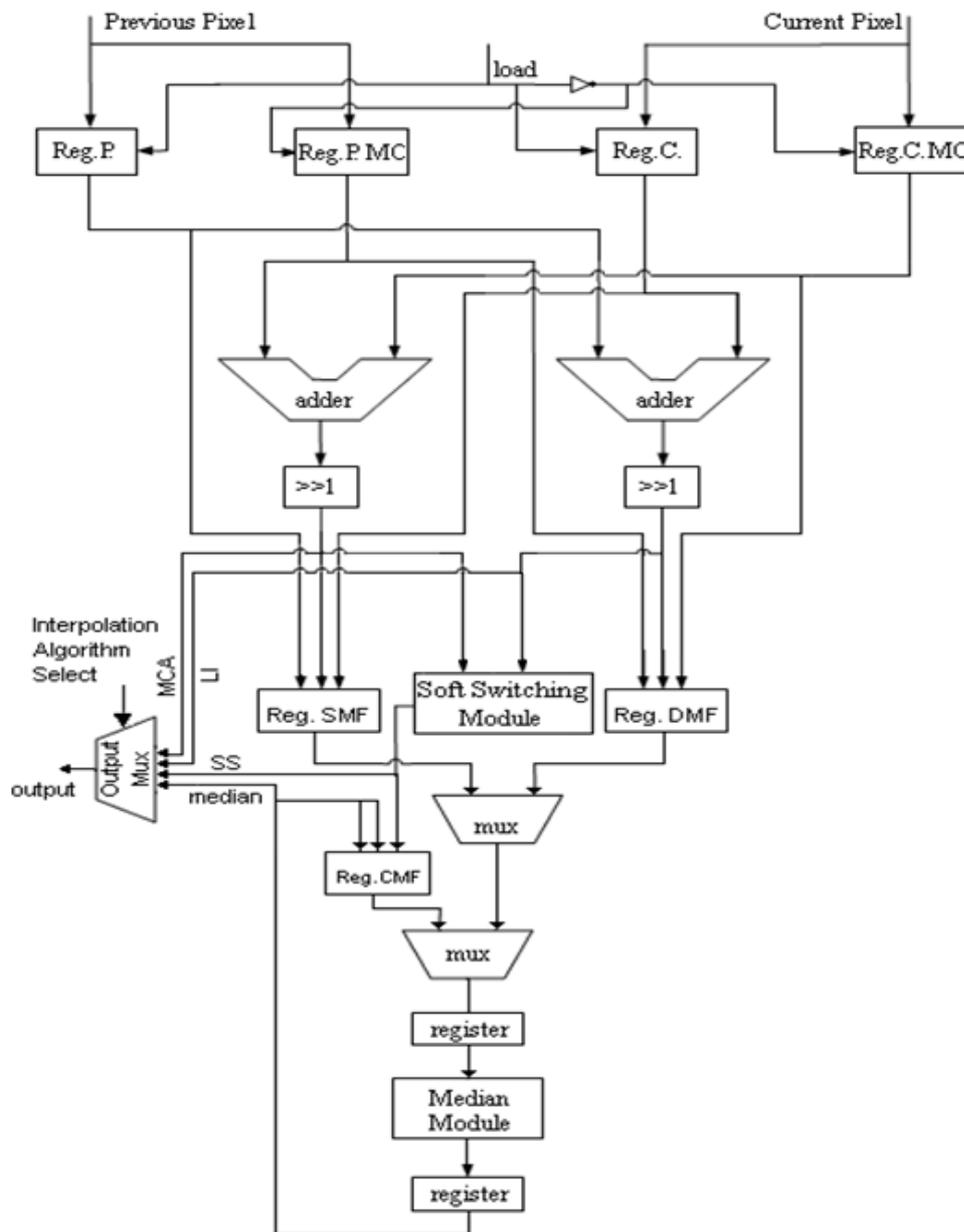
Figure 6.12 Processing element
