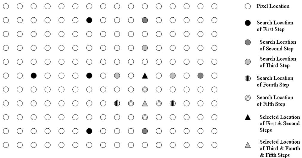
Figure 2.5 The 2D-LOGS algorithm
