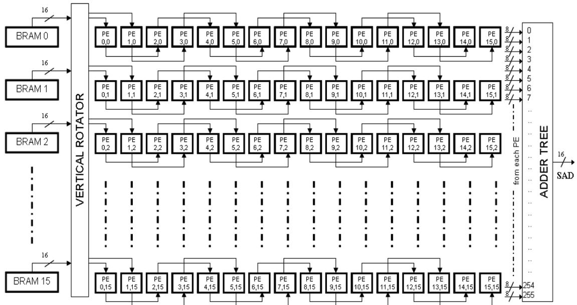
Figure 3.20 Datapath of the systolic architecture
