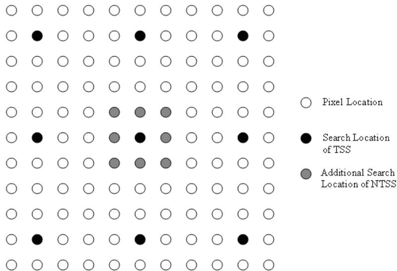
Figure 2.6 Search locations of the first step of the NTSS algorithm
