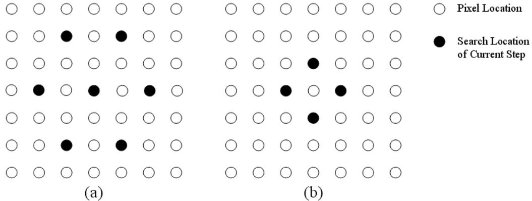
Figure 2.12 The HEXBS algorithm (a) coarse pattern, (b) fine pattern
