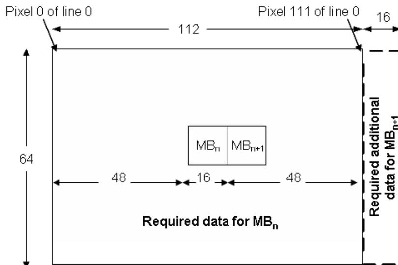
Figure 6.10 Data stored in the on-chip memory
