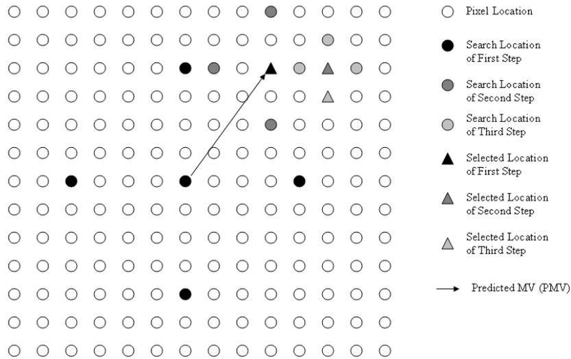
Figure 2.14 The ARPS algorithm
