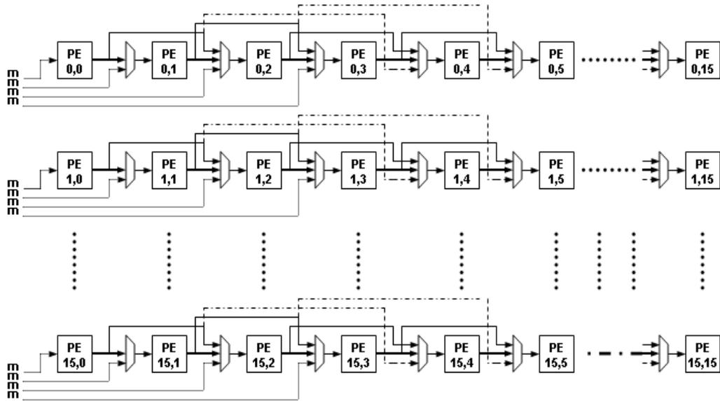
Figure 4.5 Reconfigurable systolic PE array
