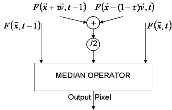
Figure 6.3 The block diagram of SMF
