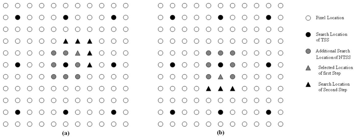
Figure 2.7 Search locations of the first and second steps of the NTSS algorithm
