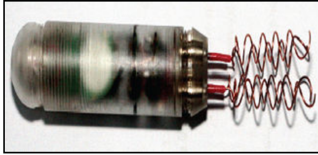
Figure 1.9: Robot prototype with four helical tails made from Shape Memory Alloy (SMA)
