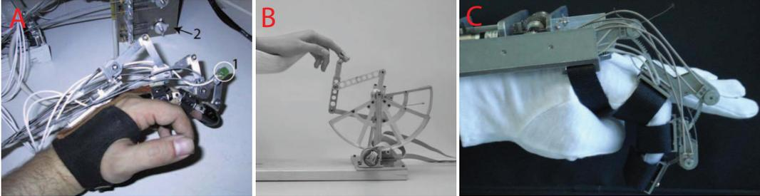
Figure 1.9: Finger exoskeletons for hand therapy: (a)Wege et al. (b)Mali et al. (c)Fu et al.
