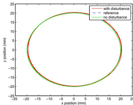
Figure 4.4: Circle tracking with/out load under impedance control
