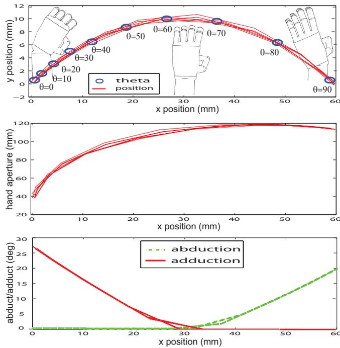
Figure 5.2: Results of the usability tests for slider crank-based end effector
