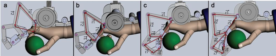
Figure 2.8: Kinematic constraint loops for joint motion of: (a)MCP (b)PIP (c)DIP
