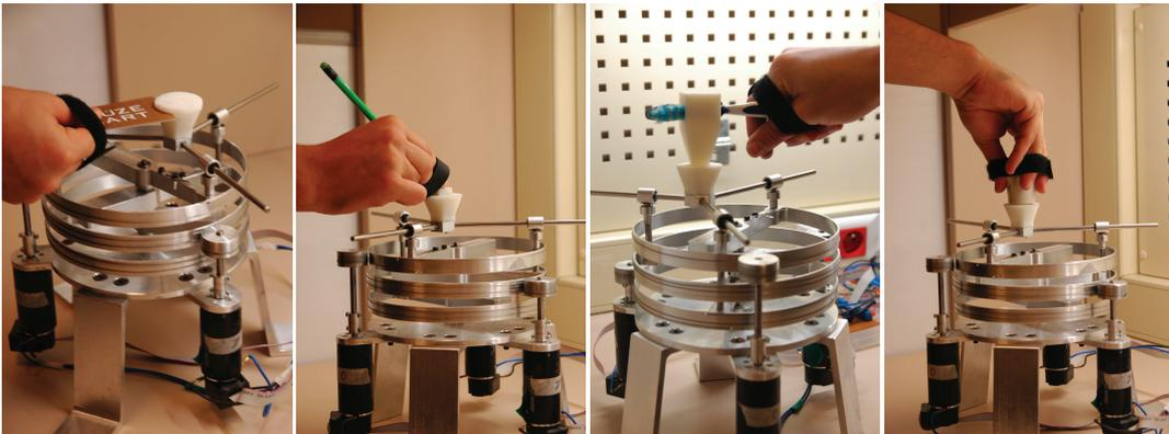
Figure 3.3: Task oriented end effectors working in horizontal plane
