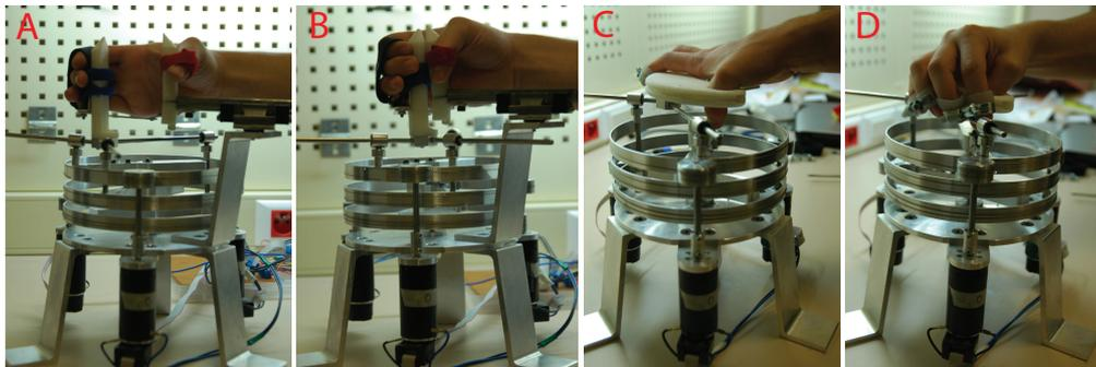
Figure 3.1: Specified motion imposing end effectors
