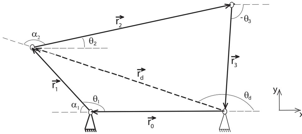
Figure 6.1: Kinematics of a four-bar mechanism
