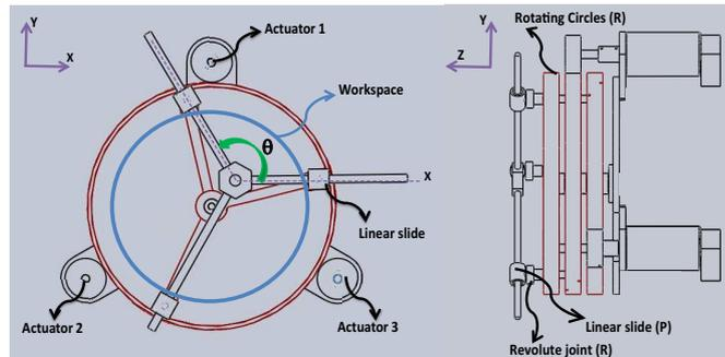
Figure 2.5: Kinematics of the 3-RRP mechanism
