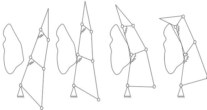
Figure 2.6: Schematic representation of the motion of the underactuated parallel kinematic chain against an obstacle
