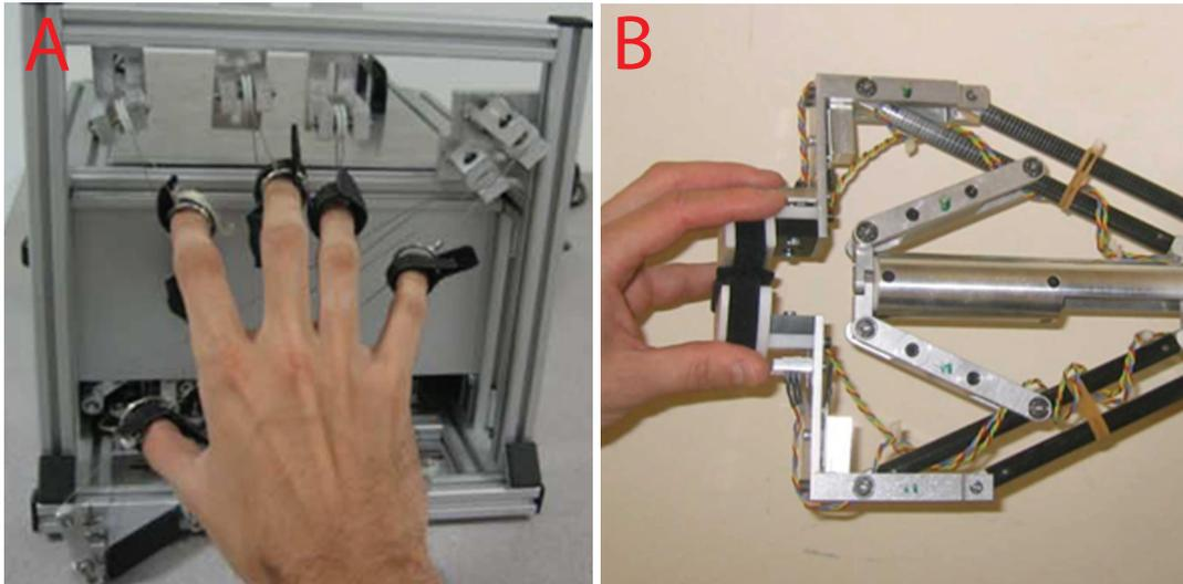
Figure 1.6: Sample end effector type robots: (a)HandCARE (b)Haptic Knob
