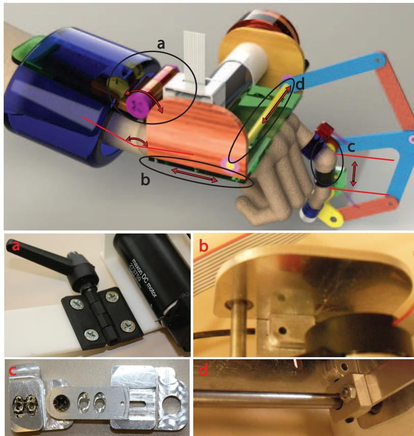
Figure 3.11: Adjustment details of the finger rehabilitation system
