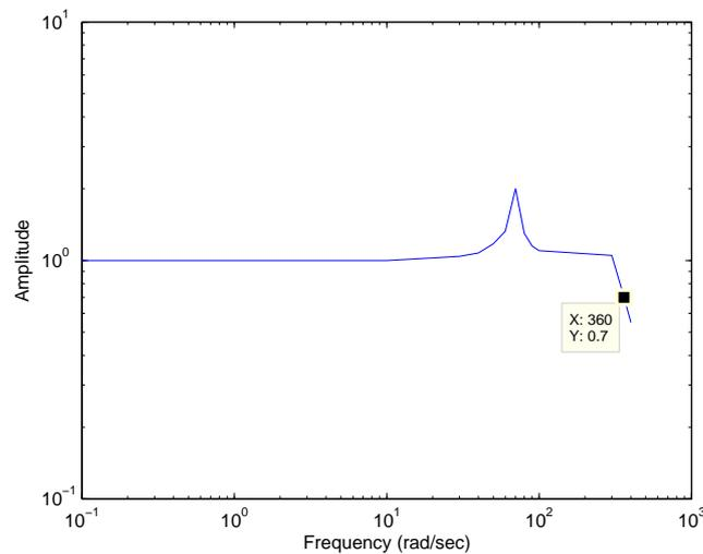
Figure 5.5: Bode magnitude diagram and bandwidth of the system
