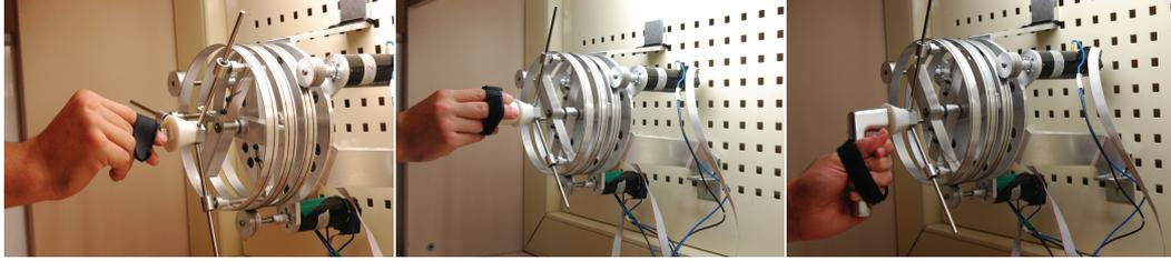
Figure 3.4: Task oriented end effectors working in vertical plane
