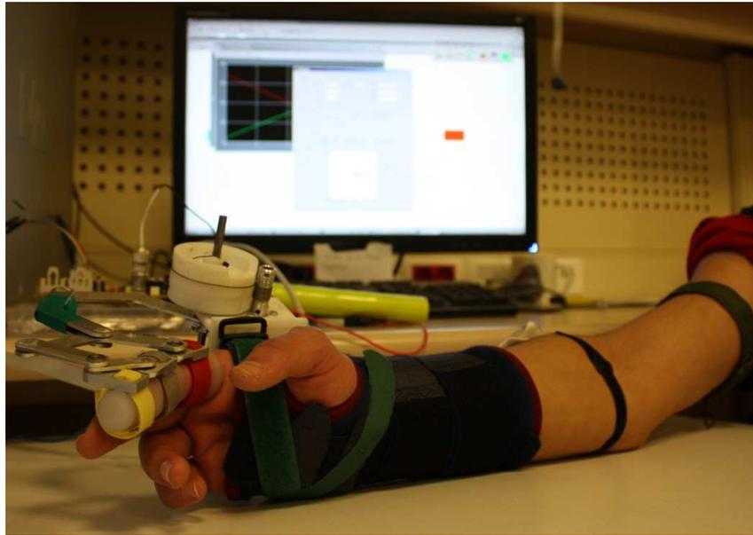
Figure 5.7: A participant attached to the finger exoskeleton device
