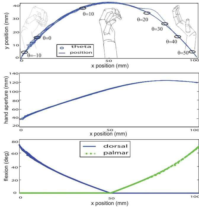
Figure 5.3: Results of the usability tests for cam-based end effector
