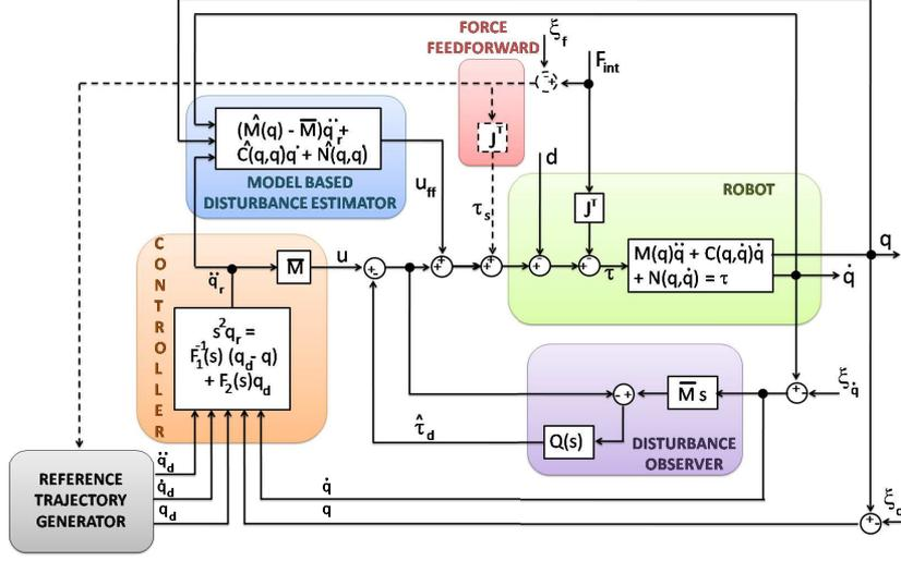
Figure 4.1: Generic model for disturbance observer based position controller
