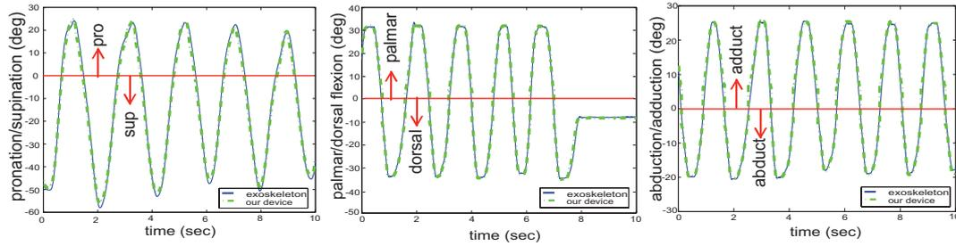
Figure 5.4: Comparison of wrist motion measurements recorded using the rehabilitation system and the SUkorpion exoskeleton
