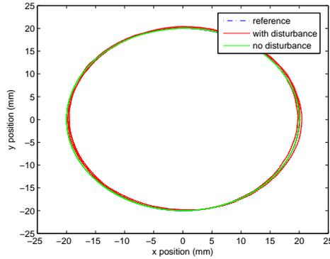
Figure 4.2: Circle tracking through PD controller
