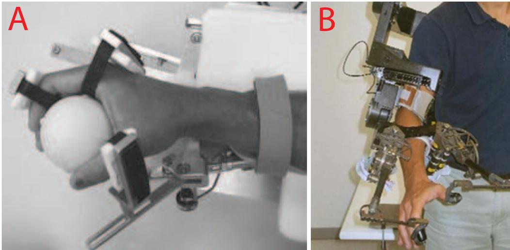
Figure 1.5: Sample exoskeleton type robots: (a)HWARD (b)PERCRO
