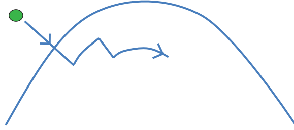
Figure 3.2.6: Trajectory of HIP on the NURBS surface. HIP is allowed to move along the parameter v and its motion along the parameter u is kept still.
