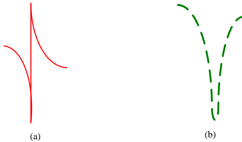
Figure 4.2 Typical rational function responses with a) real poles and b) complex poles
