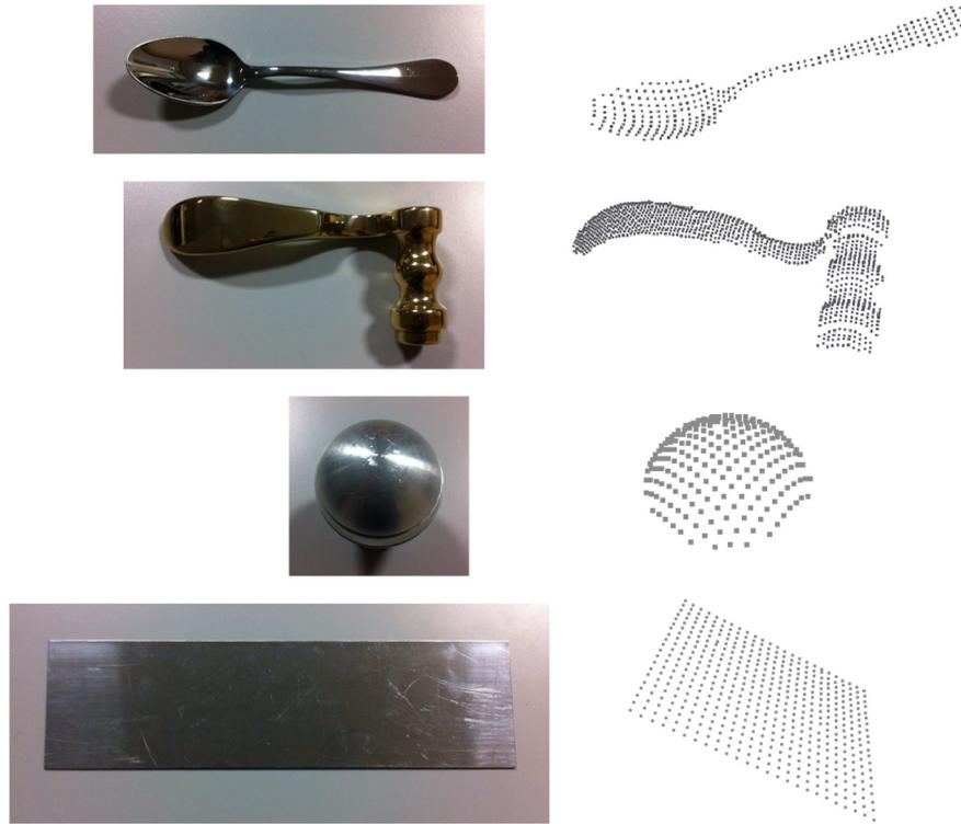
Fig. 9 3-D clouds of points digitized from specular surfaces.
