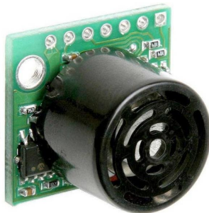
Figure 6.4: Ultrasonic Range Finder - Maxbotix LV-EZ4
