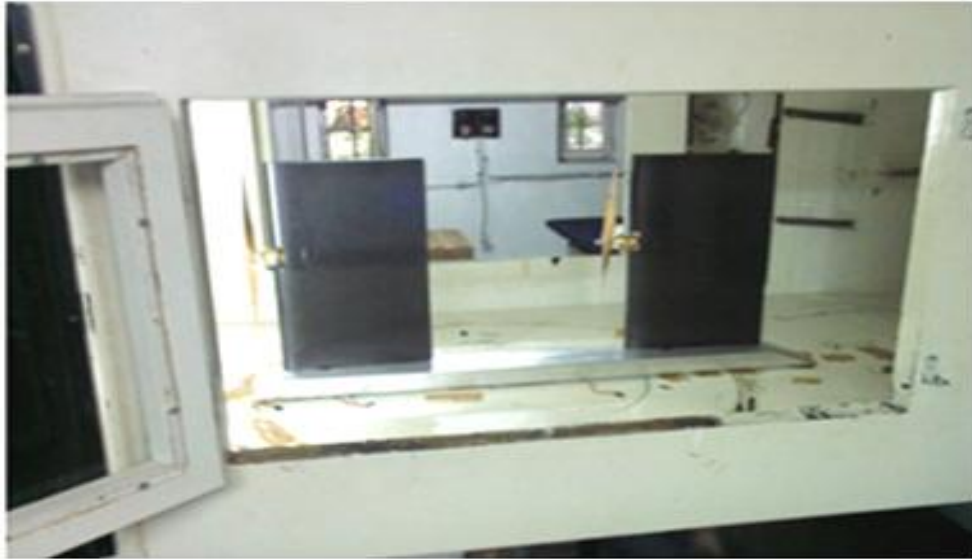
Figure 2.13: Half body model with two wings is in the wind tunnel
