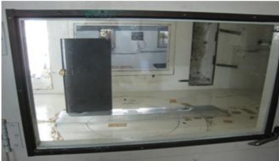
Figure 2.12: Half body model with one wing is in the wind tunnel
