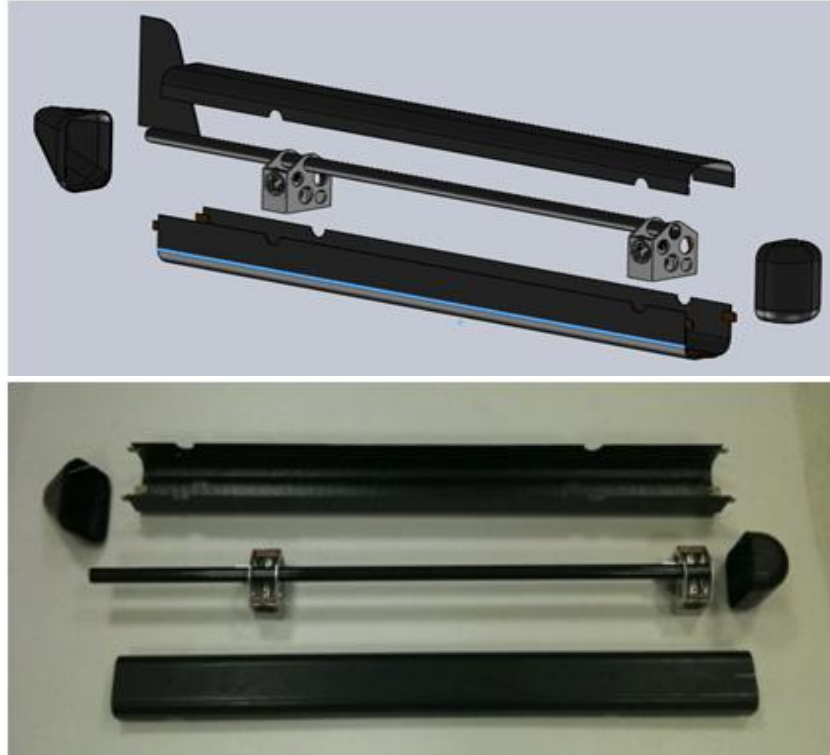
Figure 2.1: The CAD drawing and prototyping of body structure with chassis and pieces
