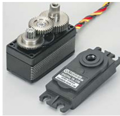
Figure 2.13: Tower Hobbies TS-170 digital servo
