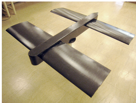
Figure 2.8: Airframe produced with carbon composite material
