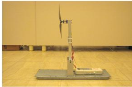
Figure 2.10: Test rig for thrust measurements
