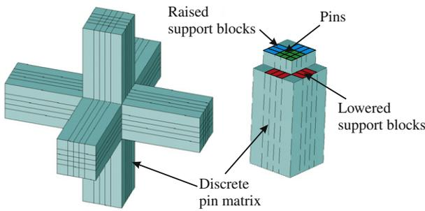
Fig. 10. 3D view of the interlocking pin configuration.
