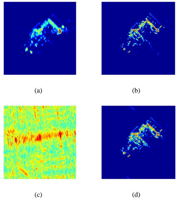
**Fig. 2.** a) Conventionally reconstructed image from data without phase errors b) Image reconstructed by sparsity-driven imaging from data without phase errors c) Conventionally reconstructed image from data corrupted by phase errors d) Image reconstructed by the proposed method from data corrupted by phase errors.
