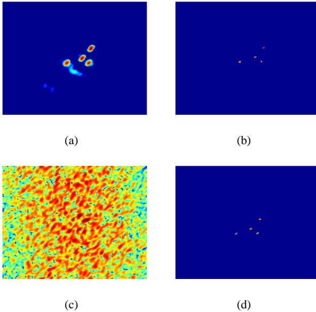
**Fig. 1.** a) Conventionally reconstructed image from data without phase errors b) Image reconstructed by sparsity-driven imaging from data without phase errors c) Conventionally reconstructed image from data corrupted by phase errors d) Image reconstructed by the proposed method from data corrupted by phase errors.
