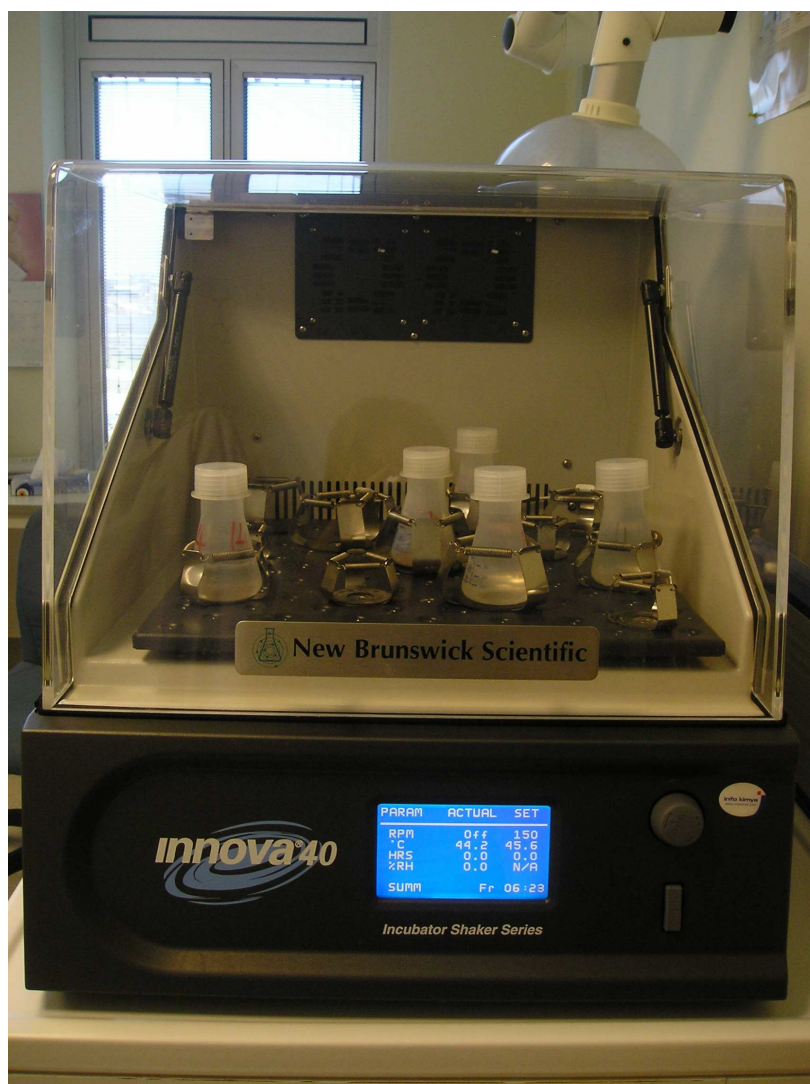
Figure 3.1. Incubator shaker used for the batch adsorption experiments
