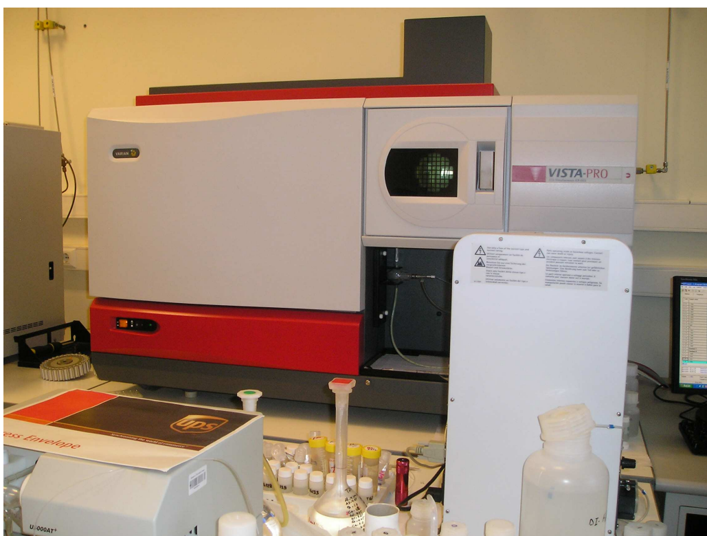
Figure 3.2. The ICP equipment used in the determination of the concentration of elements
