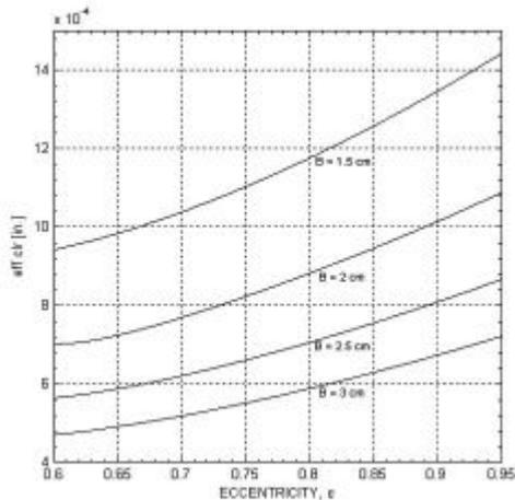
Figure (2): Effective clearance vs. Eccentricity ratio [9]
