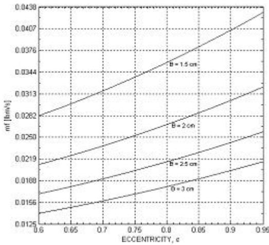
Figure (1): Mass flow rate vs. Eccentricity ratio [9]
