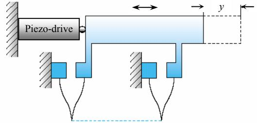
Fig. 1. Structure of a flexure piezo-stage
