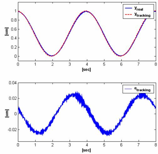
Fig. 3. Sinusoidal reference tracking with PID controller
