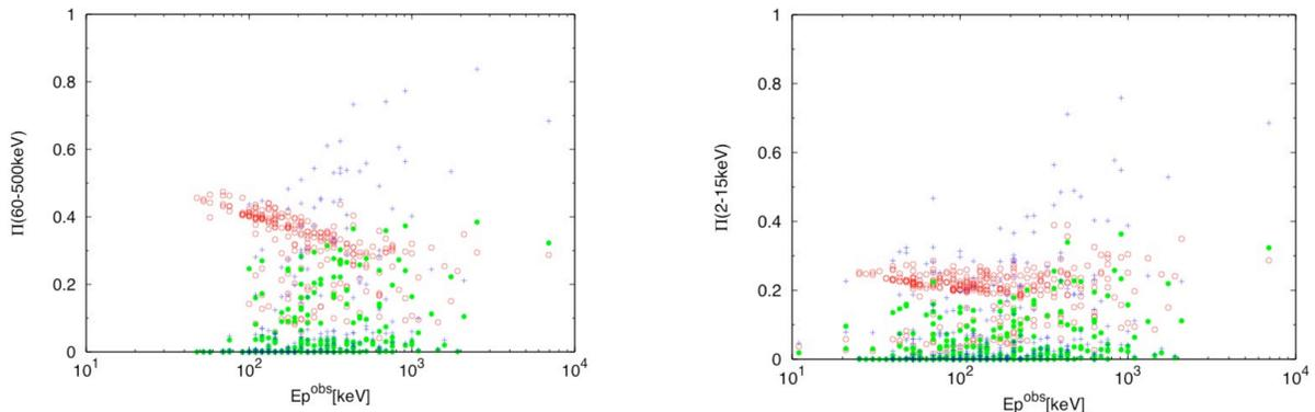
Figure 5: Simulated GRB polarization degree ( $\pi$ ) distribution for three models: Synchrotron emission in ordered magnetic fields (red), synchrotron emission in random fields (green), and Compton drag (blue). Left: 60-500 keV; Right: 2-15 keV. From [13].
