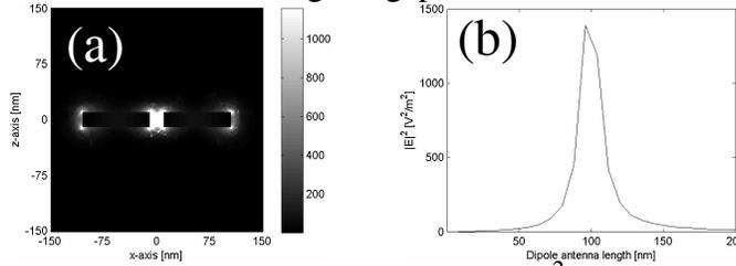
**Figure 2.** (a) The intensity distribution,  $|E(x, y=0, z)|^2$  on the  $x$ - $z$  plane for a dipole antenna at a wavelength of 850 nm for  $L= 110$ ,  $T= 20$ ,  $W= 20$ , and  $G= 20$  nm, and (b) The intensity at the center of the gap  $|E(x=0, y=0, z=0)|^2$  is plotted for various  $L$  at  $\lambda = 850$  nm.
