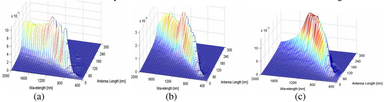
**Figure 4.** The intensity as a function of wavelength and antenna length for: (a)  $T=10$ ,  $W=10$ , and  $G=20$  nm, (b)  $T=20$ ,  $W=20$ , and  $G=20$  nm, and (c)  $T=50$ ,  $W=50$ , and  $G=20$  nm.
