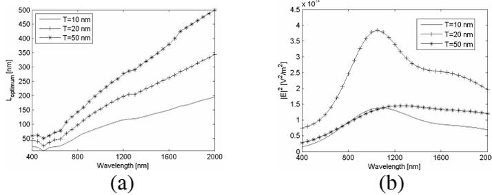
**Figure 5.** (a) Optimum gold dipole antenna length as a function of wavelength, (b) Optimum intensity values  $|E(x, y=0, z)|^2$  for optimum antenna lengths as a function of wavelength.
