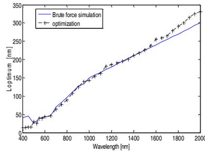
**Figure 8.** Comparison of the optimization result for a dipole antenna using the SQP method and brute-force simulations.
