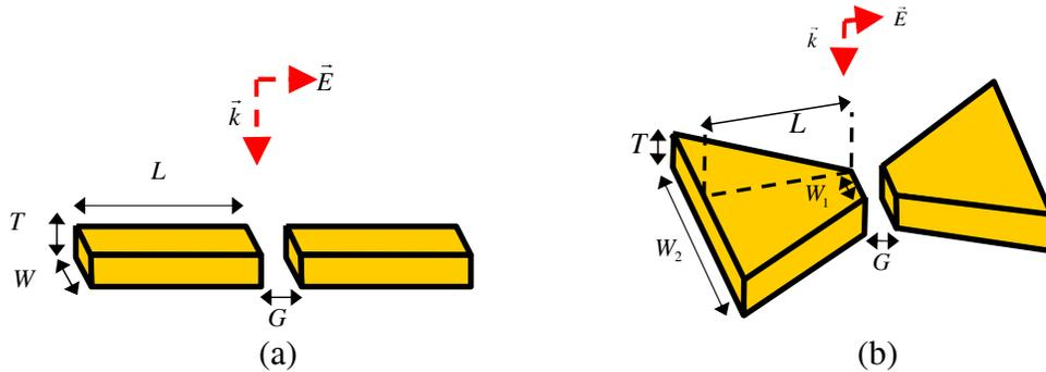
**Figure 1.** A schematic illustration of a (a) dipole and (b) bow-tie antenna, and their dimensions. The antennas are illuminated with incident electromagnetic radiation shown with  $\vec{E}$ .
