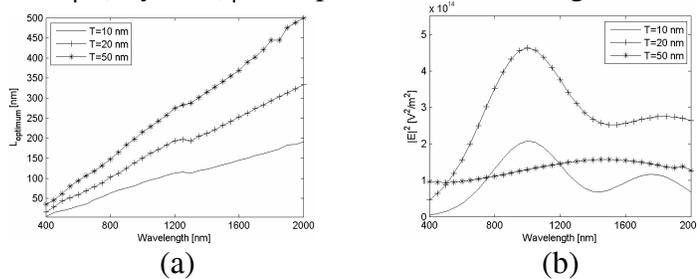
**Figure 6.** (a) Optimum silver dipole antenna lengths as a function of wavelength, (b) Optimum intensity values  $|E(x, y=0, z)|^2$  for optimum antenna lengths as a function of wavelength.
