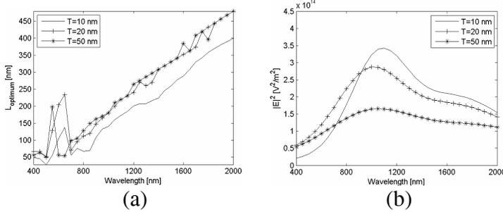
**Figure 7.** (a) Optimum gold bow-tie antenna lengths as a function of wavelength, (b) Optimum intensity values  $|E(x, y=0, z)|^2$  for optimum antenna length as a function of wavelength.
