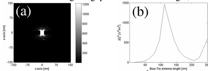
**Figure 3.** (a) The intensity distribution,  $|E(x, y=0, z)|^2$  on the  $x$ - $z$  plane for a bow-tie antenna at a wavelength of 850 nm for  $L= 100$ ,  $T= 20$ ,  $W_1= 20$ ,  $W_2= 220$ , and  $G= 20$  nm, and (b) The intensity at the center of the gap  $|E(x=0, y=0, z=0)|^2$  is plotted for various  $L$ , at a  $\lambda = 850$  nm.
