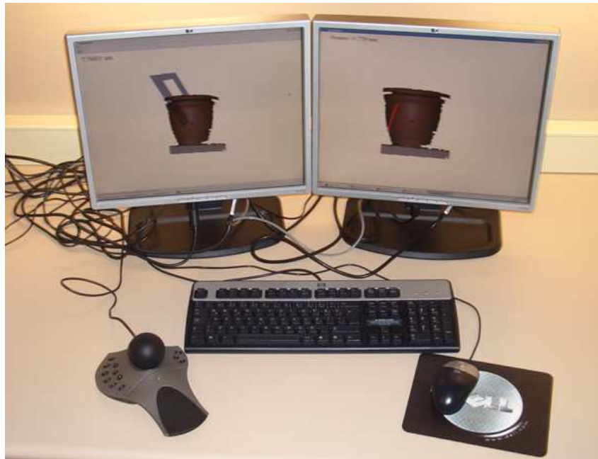
Figure 5.1: System setup showing the spaceball on the left (non-dominant hand) and the mouse on the right (dominant hand)
