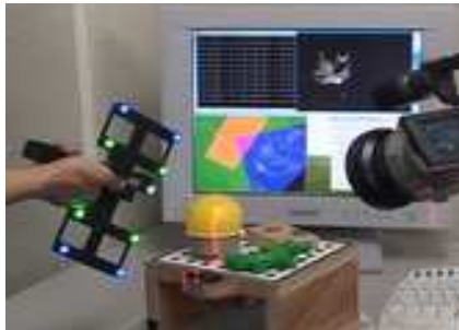
Figure 3.5: A computer vision based handheld 3D scanning prototype.
