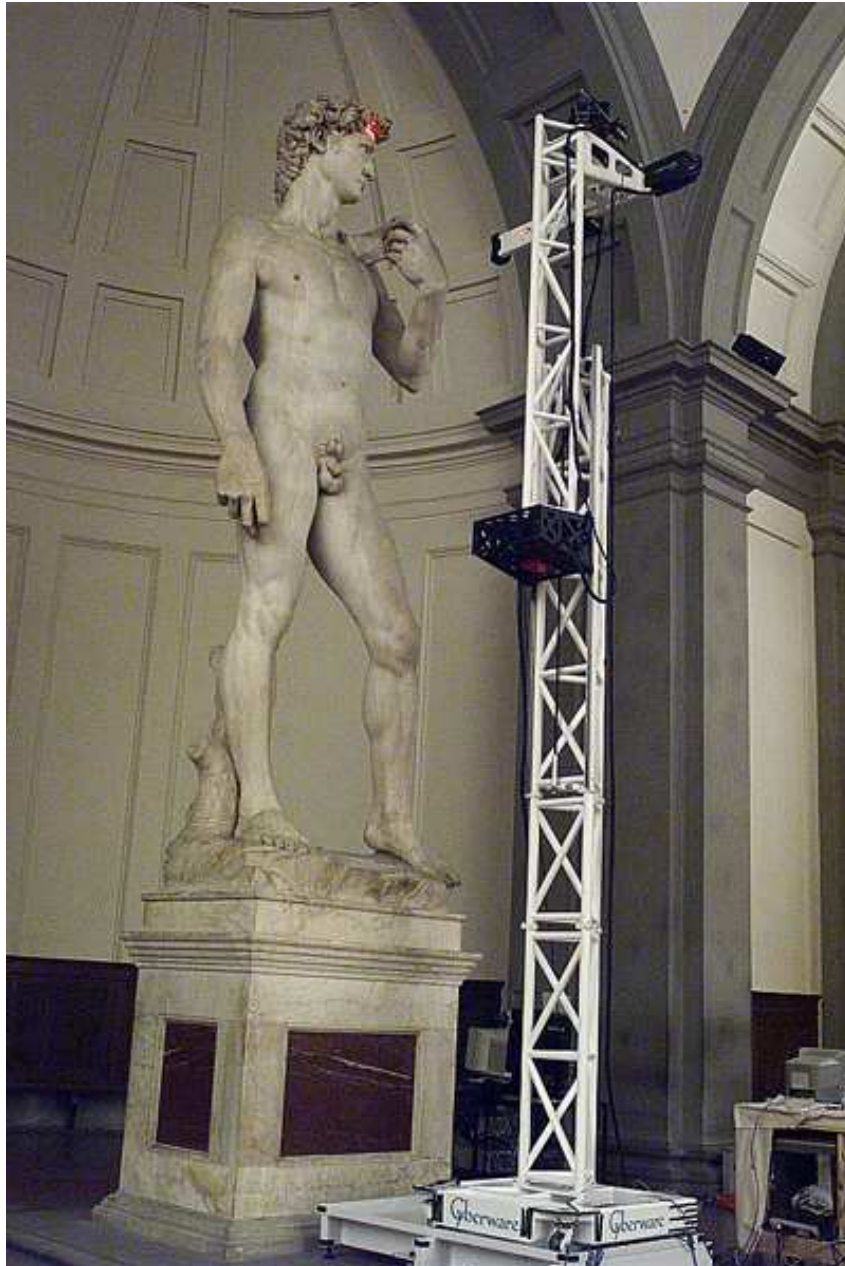
Figure 3.3: The scanner mounted on a moving platform to scan the head of the David statue as part of the Digital Michelangelo Project.
