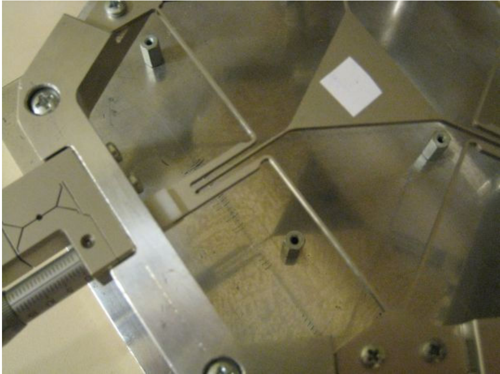
Figure 5.7 The actuator mounting and the dot on the triangular stage
