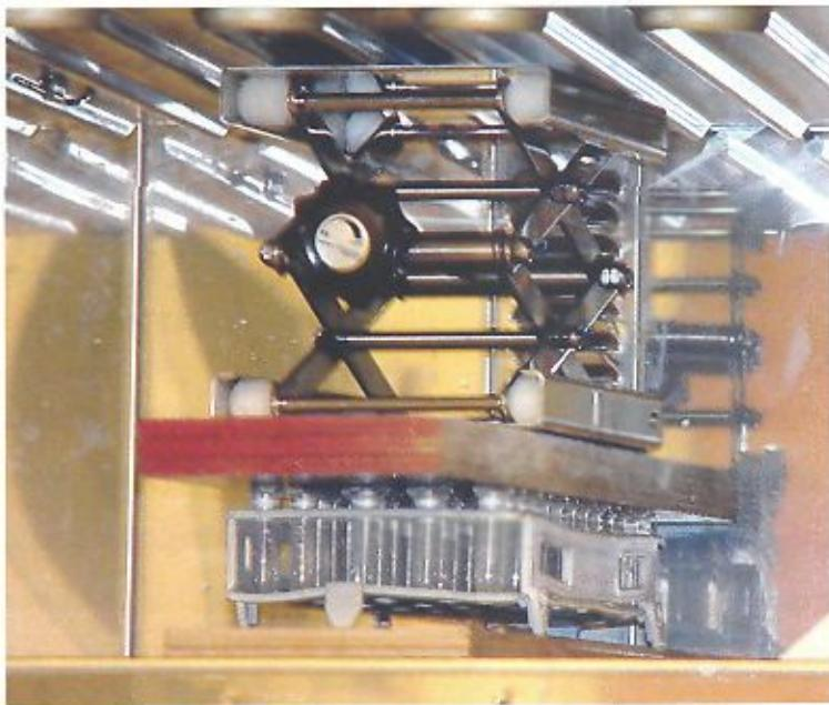
Figure 15: Set-up used to restrain caps during the course of oxidation.
