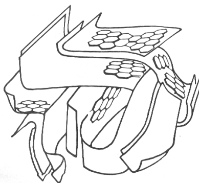
Figure 2.4. Schematic representation of graphite sheets [11].
