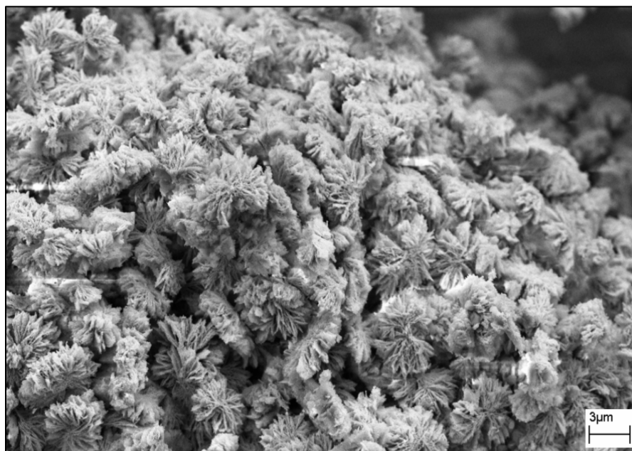
Figure 4.16. SEM image of HF washed raw natural zeolite.
