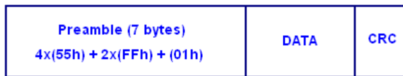
Figure 3.19 Wireless communication packet structure.
