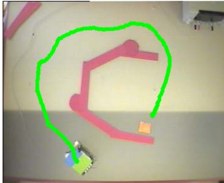
Figure 4.12 Solution to the problem when goal is too close to an obstacle.
