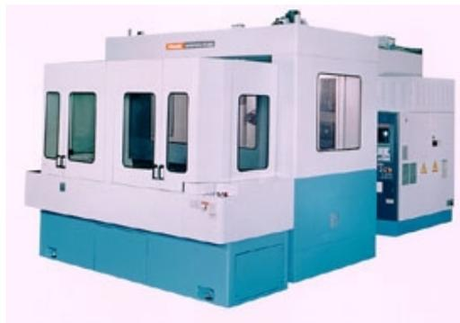
Figure 3.1 Machining Center
