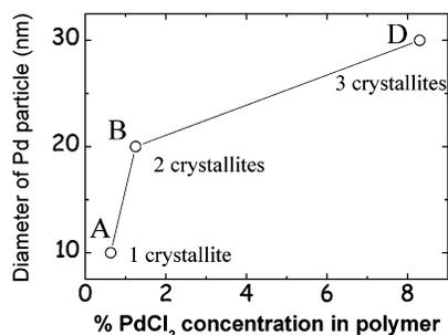
**Figure 6.** Pd particle size as a function of PdCl<sub>2</sub> concentration inside spinning solution.
