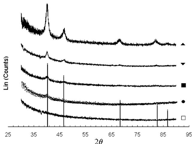
**Figure 3.** X-ray diffraction peaks of mat PAN with (□) 5.4 mol % AA and 1.25% PdCl<sub>2</sub> before the reduction process, (●) 5.4 mol % AA and 0.63% PdCl<sub>2</sub> after the reduction process, (■) 5.4 mol % AA and 1.25% PdCl<sub>2</sub> after the reduction process, (▼) 8.1 mol % AA and 1.25% PdCl<sub>2</sub> after the reduction process, and (▲) 5.4 mol % AA and 8.3% PdCl<sub>2</sub> after the reduction process.
