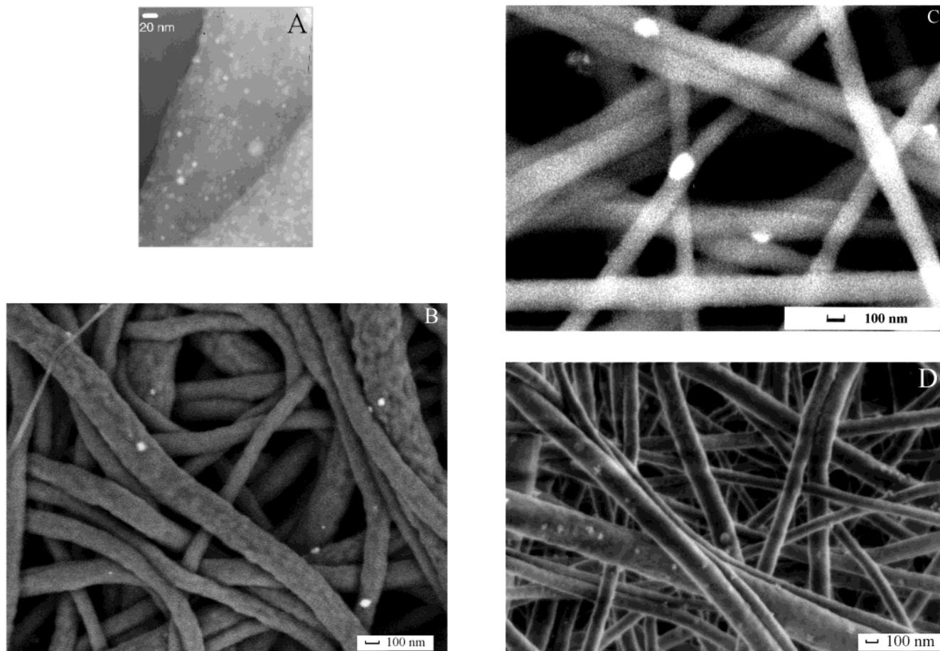
**Figure 4.** Electron microscope images of PAN-AA fibers with generated Pd nanoparticles: (a) sample A, (b) sample B, (c) sample C, and (d) sample D. Sample A is magnified 300K times and the others 50K times.
