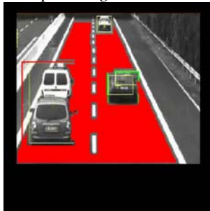
Asphalt segmentation and car detection
