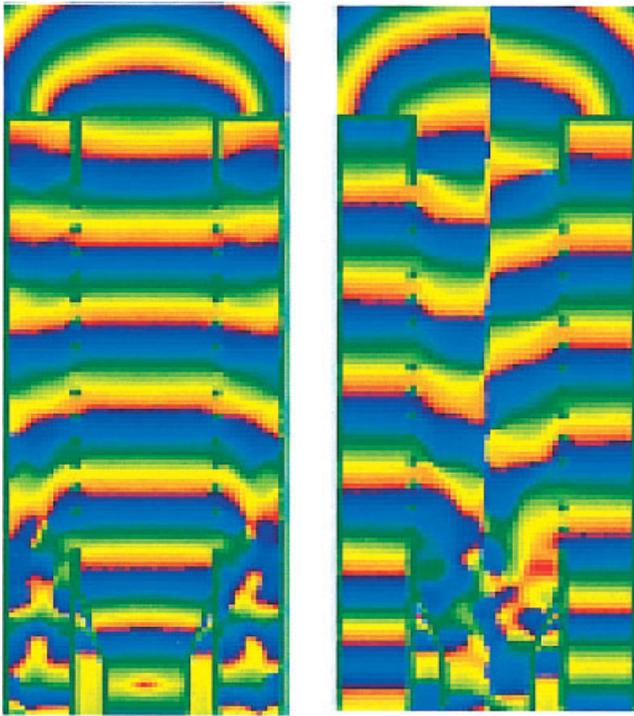
**Figure 8** Phase distribution in the cross section of the mode coupler for sum (left) and difference (right) patterns. [Color figure can be viewed in the online issue, which is available at [www.interscience.wiley.com](http://www.interscience.wiley.com)]
