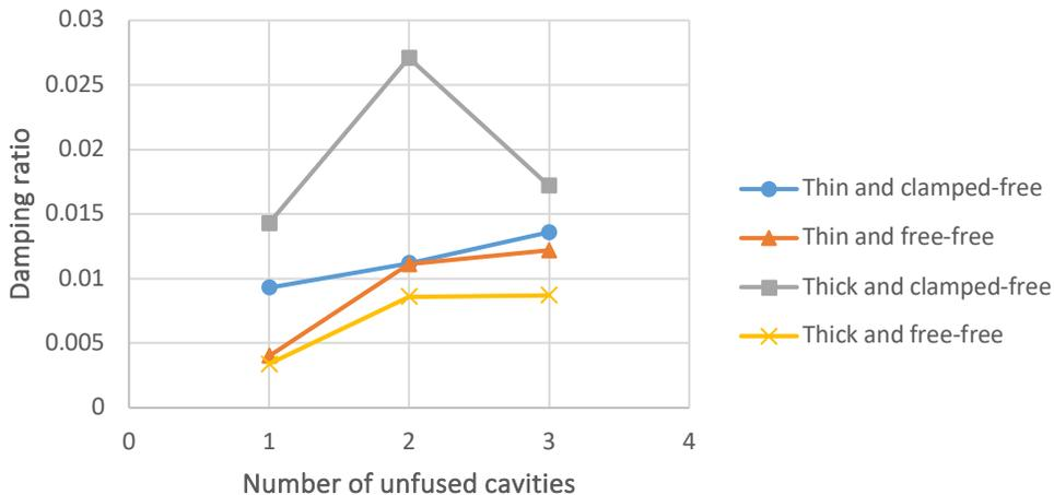
**Figure 5.** Effects of variation in the number of cavities on the damping ratio
