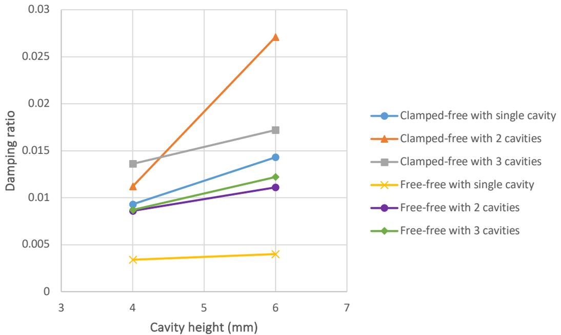
**Figure 6.** Effects of variation in the cavity height on the damping performance
