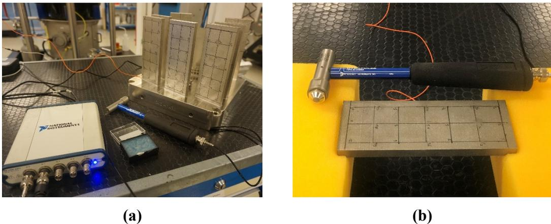
**Figure 3. a) Clamped-free and b) free-free modal test setups**
