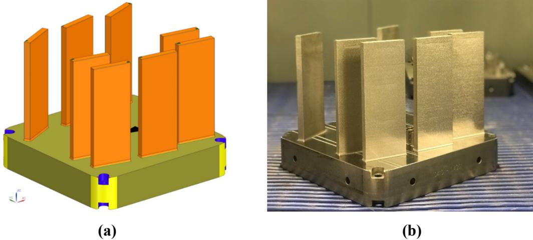
**Figure 2. a) Specimens placed on the build plate and b) Fabricated specimens**
