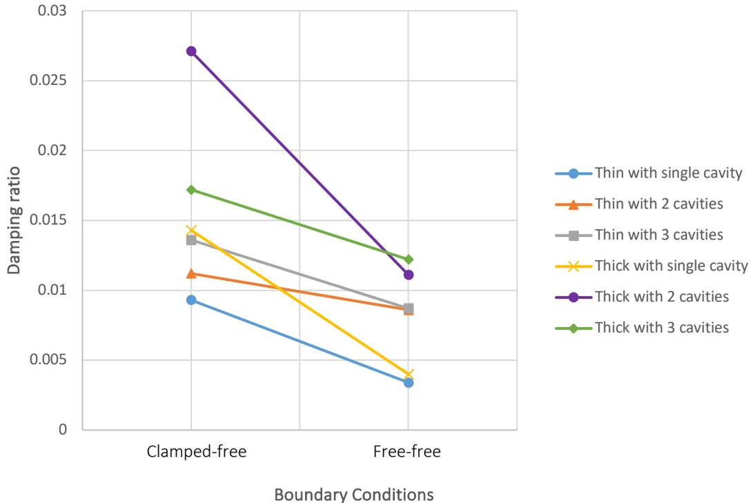
**Figure 7.** Effects of boundary conditions on the damping performance
