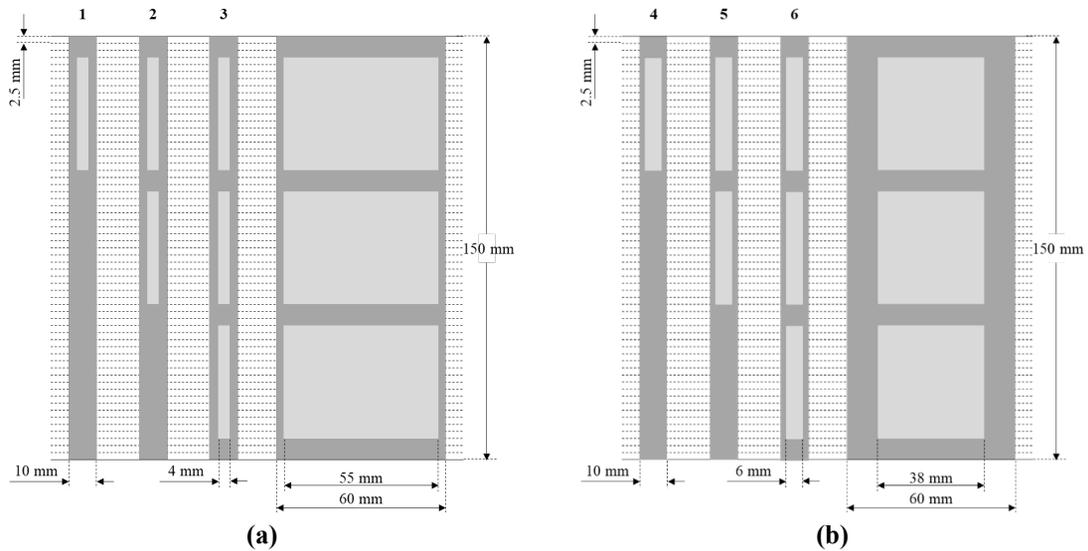
**Figure 1.** Specimens with a) thin unfused cavities and b) thick unfused cavities
