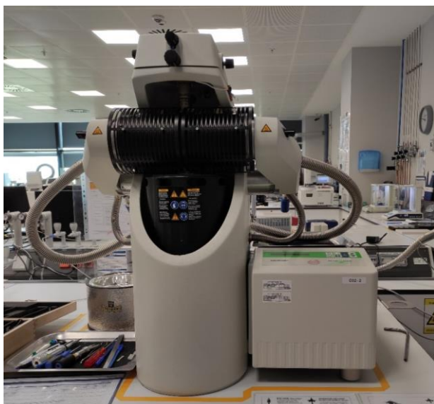
Figure 11. Dynamic Mechanical Analysis (DMA) for T_g measurements
