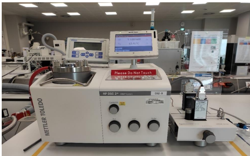
Figure 7. High Pressure Differential Calorimetry (HP-DSC) for cure kinetic studies
