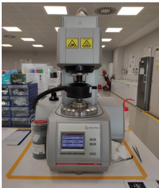
Figure 10. Rheometer for cure kinetic studies
