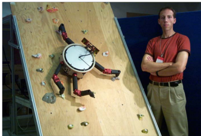
Figure 2.2 A free climbing robot, LEMUR.
