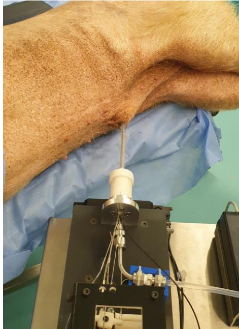
Figure 5.1. Testing the diameter of the probe and capability of control system in penetrating and advancing into the urinary system of pig.
