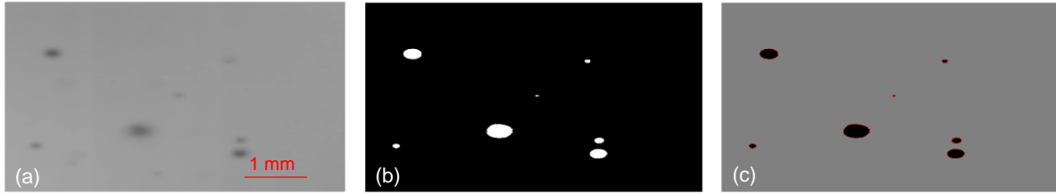
Figure 4.5. Droplet recognition during the image processing using MATLAB™ 2018a software. (a) Raw image, (b) Threshold image, (C) Final processed image with boundaries for each recognized image.
