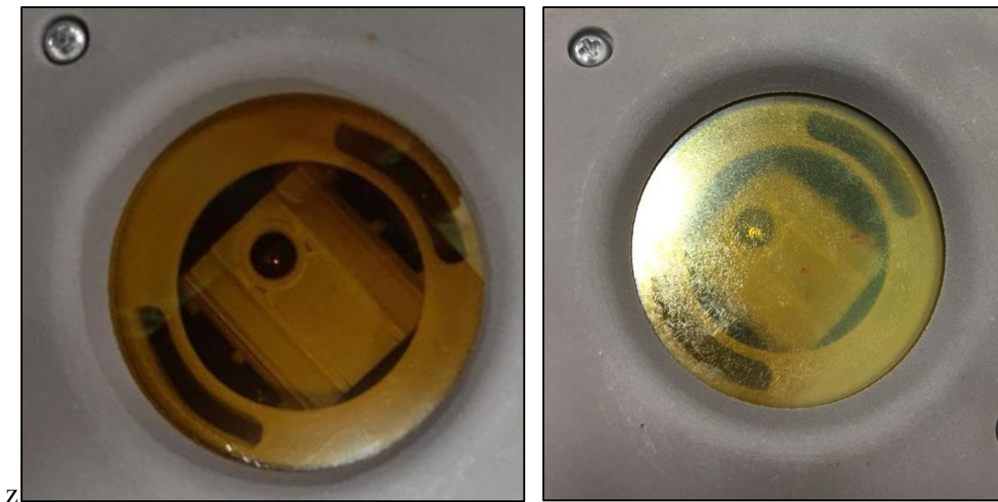
Figure 41 Left, protective housing window before the process. Right, contaminated window after the process.
