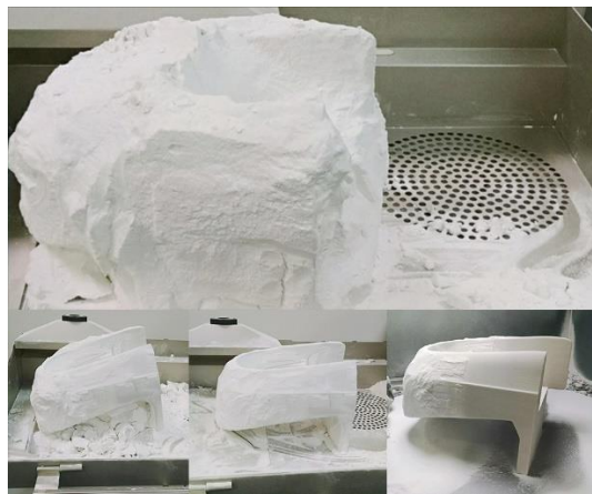
Figure 2 Powder aggregates from the build cake [10]
