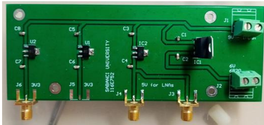
Figure 3.55 Voltage regulator for repeater hardware
