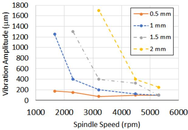
Fig. 7: Variation of vibration x-y amplitude.
