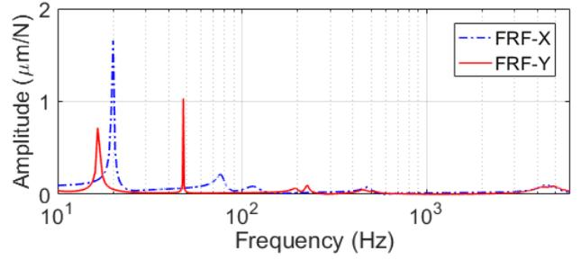
Fig. 3: FRF in X and Y directions measured at the tool tip.
