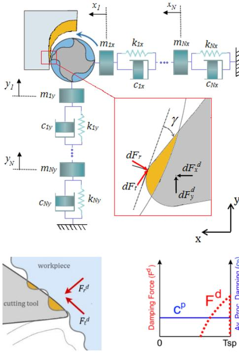
Fig. 2: Process damping effect in milling (a) Multi-mode milling (b) tool – workpiece interaction (c) Damping energy balance [Tunc et al. 2018].
