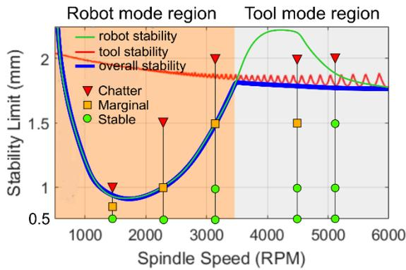
Fig. 4: Stability diagram for the robotic milling system.
