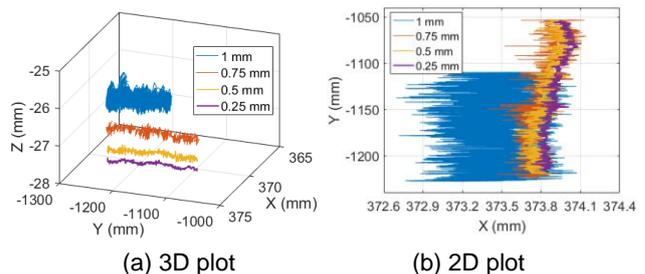
Fig. 6: Laser tracker measurement at 1660 rpm.
