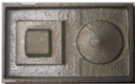
(a) Example part manufactured by AWJM [Popan, A. 2015].
