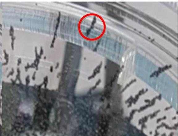
Figure 3.4 Iron dust particle experiments. a) under uniform magnetic field, dusts particles cluster near the magnets and the edges, b) under non-uniform magnetic field dusts begin to distribute throughout the plate, when the system is operational c) dusts align successively, d) lift e) roll and change direction in their own axis, f) lift again.
