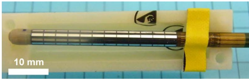
Figure 2.3: CMUT-based ten facets HICU catheter prototype [46].
